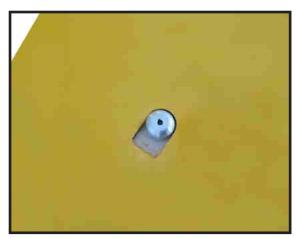
It is best to operate the aero-tow release mechanism using a momentary switch mounted on the joystick. Th servo travel must be set accordingly.
