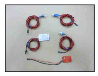
Two white lights for cowling and rudder, the green light for right wing tip, and the red light for left wing tip. They are designed to operate on voltages 12 volts. Connect four lights into switch circuit so that optional the different flashes mode.
