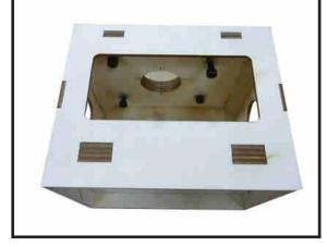
Attach the motor to the front of the electric motor box using four 4mm blind nut, four M6x35mm hex head bolts to secure the motor. Please see picture shown.
