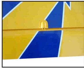
Use canopy glue to attach the cover to the wing. Use low-tack tape to keep the cover in position until the adhesive fully cures.
