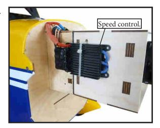
the motor box using two-sided tape and tie wraps. Connect the appropriate leads from the speed control to the motor. Make sure the leads will not interfere with the operation of the motor.
