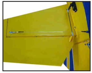
INSTALLING THE WING STRUT
