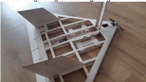
Front of rudder has both sides balsa strip precut
