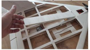
Deck rotates around rest of 2mm control rod
