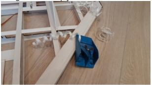
Sand balsa LE in shape (5\*15mm strips) Capstrips are approx 10 to 12mm wide
