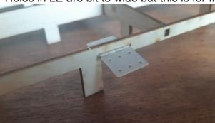
Hinges will fit in ply TE and balsa LE for rudder
