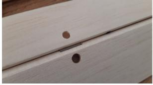
Servo comes locked partly in the spar and gluedHoles for glueing and fixing hinges
