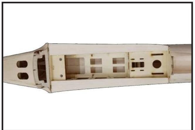
Fitting the wing to the fuselage and adjust the SH13 sheet so that there is not gap at interface. Then, add CA glue to keep fixed SH13 (Photo 5).
