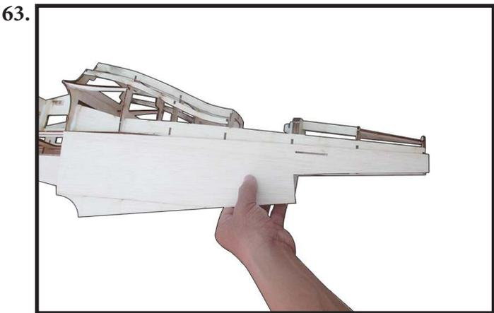
Bend the balsa sheet go to the curve of top area. Then, add CA glue and use the finger at this place until the glue dries as photo shown (Photo 64). Do the same for the other half of the top area, so that the balsa sheet keep fixed fuselage.
