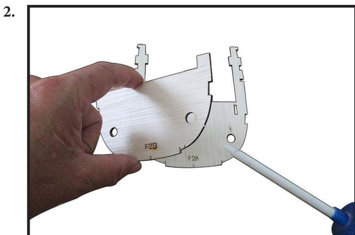
As photo shown (photo 3), you can use 100% epoxy glue. And then, use heavy flat thing pressed on F2 block until the glue dries. Or you can use CA glue at some places to help holding them temporarily. At this time, you can do next step to save more time while waiting epoxy dries.
