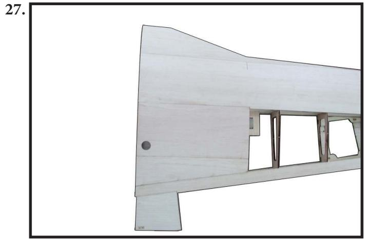
Reinforced W37 to sheeting at the wheel area as photo shown (photo 25,26,27). Then, step by step cover sheet one after another in order W31-W33-W35-W38 for top of wing.
