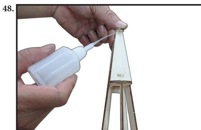
Locate and assemble F3B and F4B to fuselage by CA glue as photo shown (photo 49).
