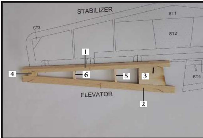
Remove nail Stabilizer and Elevator after glue dries (Photo 4).
