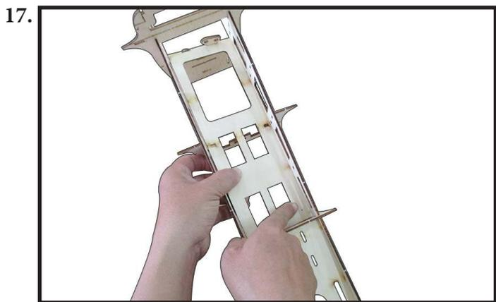
Locate and assemble F13 to fuselage by CA glue as photo shown (photo 21,22).
