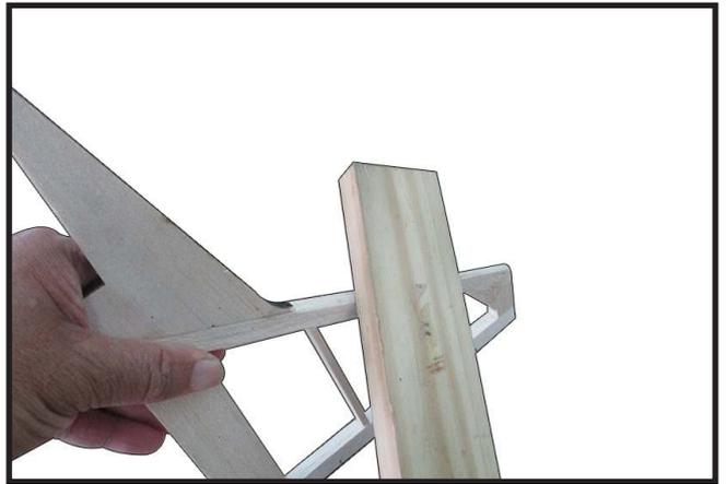
Locate position of paper hinge for Fin and Rudder as plan. Then, sawn the slot ( for 3 hinges) by the blade tool. First, assemble 3 paper hinges to Fin. Then, link to Rudder. Finish assemble Fin and Rudder (Photo 6).
