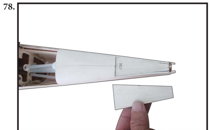
Some place can't bend by balsa sheet because curve shape is too short, the balsa sheet will break easily. So the balsa block is inserted. Then, cut down the balsa block to shaping curve and sanding (photo 79, 80, 81).
