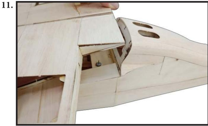
Put fiberglass part on wing to locate place of holes. Then, drill two holes on the special fiberglass part. (Photo 15,16).
