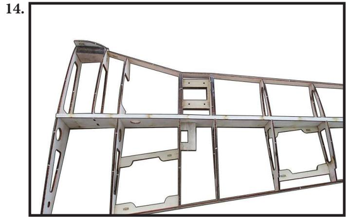
Locate and assemble wing tube. Light sanding the wing tube to it can through to holes easily as photo shown (photo 15).
