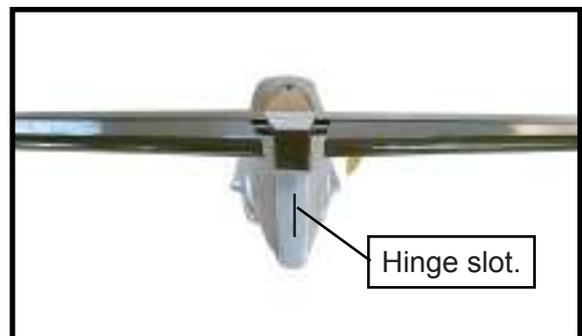
3) While holding the vertical stabilizer firmly in place, use a pen and draw a line on each side of the vertical stabilizer where it meets the top of the fuselage.
