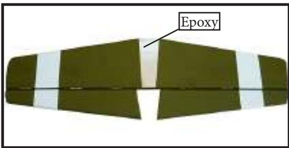
7) When you are sure that everything is aligned correctly, mix up a generous amount of 30 Minute Epoxy. Apply a thin layer to the top and bottom of the stabilizer mounting area and to the stabilizer mounting platform sides in the fuselage. Slide the stabilizer in place and realign. Double check all of your measurements once more before the epoxy cures. Hold the stabilizer in place with T-pins or masking tape and remove any excess epoxy using a paper towel and rubbing alcohol.
