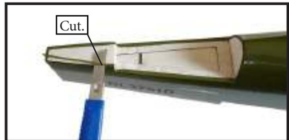
3) Slide the stabilizer into place in the precut slot in the rear of the fuselage. The stabilizer should be pushed firmly against the front of the slot.
