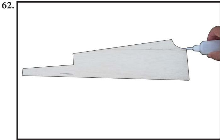
Put the sheet at top area and toward rear of fuselage as photo shown (photo 63).
