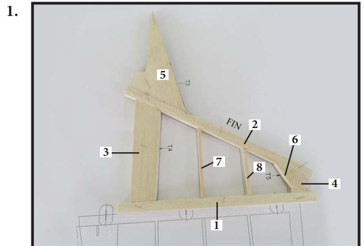
Locate and assemble the Rudder as the plan. Step by step do it one after another in order 1-7. Use the nail to plug in keep the rib on the paper plan and add CA glue. Remove nail after glue dries (Photo 2).
