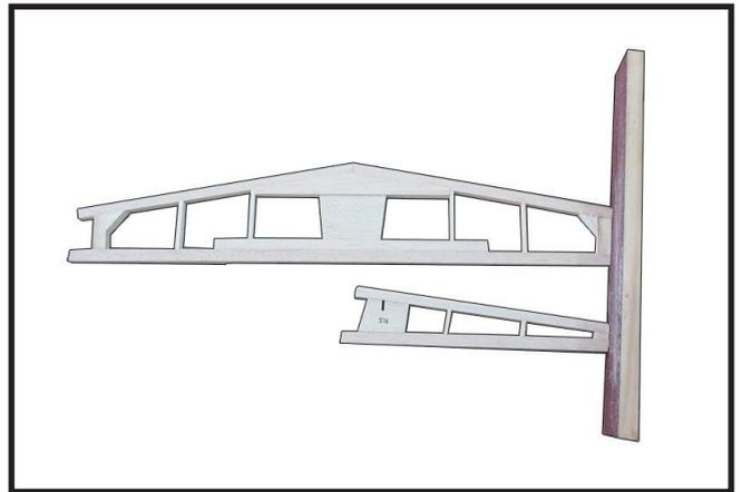
Rounded the edge around of Stabilizer and Elevator by sanding tool (Photo 6).
