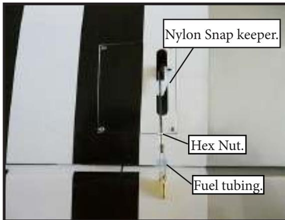
Use a felt tip pen to mark the wire where it crosses the hole. Use a pair of pliers to put a sharp 90-degree bend in the wire at the mark.
