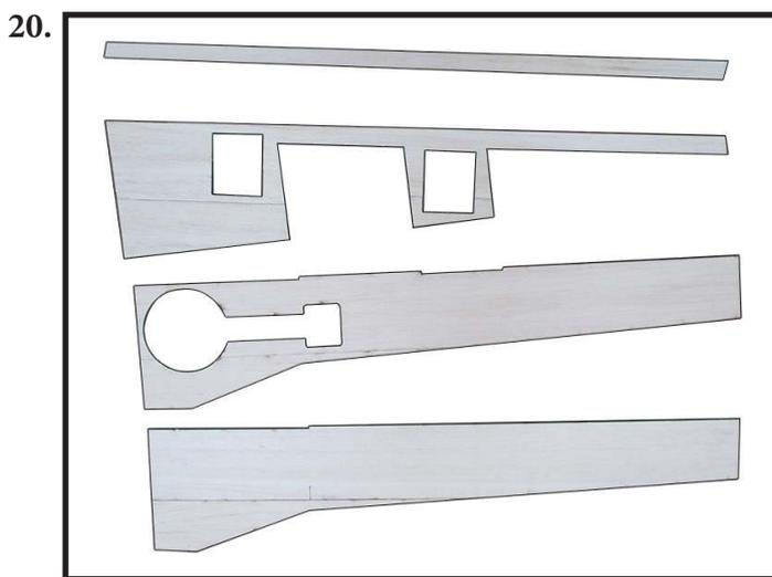
Cover sheet for wing. First, covering the bottom of wing. Step by step do it one after another in order W32-W33-W34 as (photo 21).
