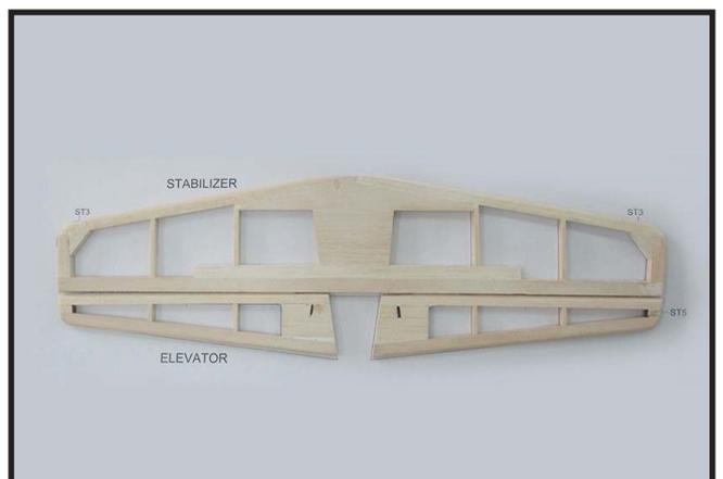
Locate position of metal elevator joiner wire (Photo 8). Then, drill the ( $\varnothing$  3mm) round well inside Elevator. The deep value of well is equal to dimension of the wire part which bends 90 degree angle like a hook. (Photo 9).
