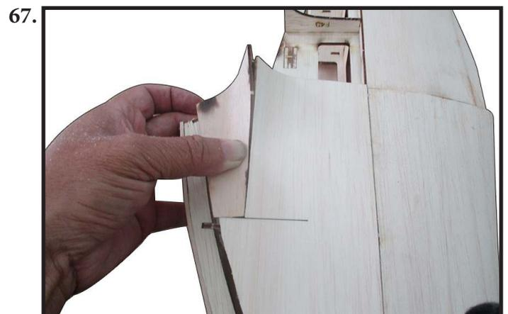
Put the sheet SH3 at forward area of fuselage as photo shown (photo 68). Then, add CA glue and use the finger at this place until the glue dries. Do the same for the other half.
