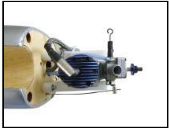
8) Connect the Z-bend in the 450mm throttle pushrod to the outer hole of the throttle servo arm.
