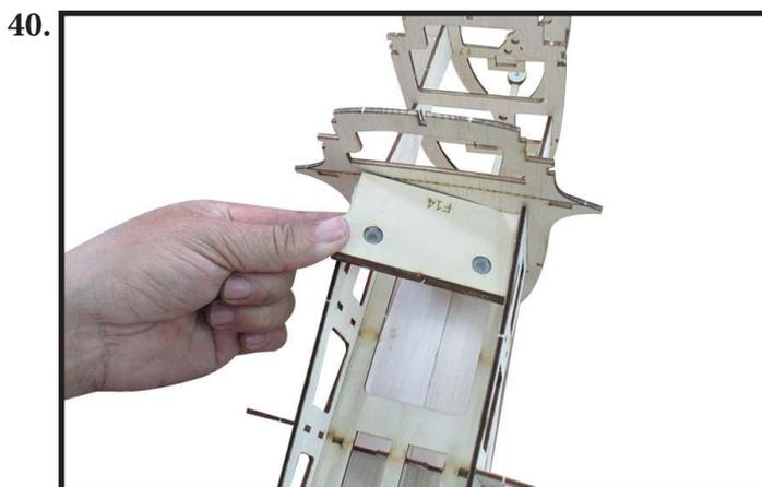
Locate and assemble F21 to fuselage by CA glue as photo shown (photo 41).
