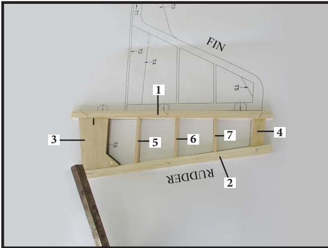
Cut off the excess balsa wood part and sanding smooth and flat the edge. Then, rounded the edge around of Fin and Rudder by sanding tool (Photo 3,4,5).
