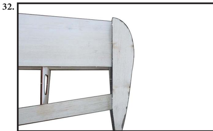
Locate and assemble W12 (wing tip) by epoxy glue as photo shown (photo 30).
