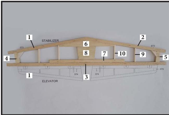
Locate and assemble the Elevator as the plan. Step by step do it one after another in order 1-6. Use the nail to plug in keep the rib on the paper plan and add CA glue. (Photo 3).
