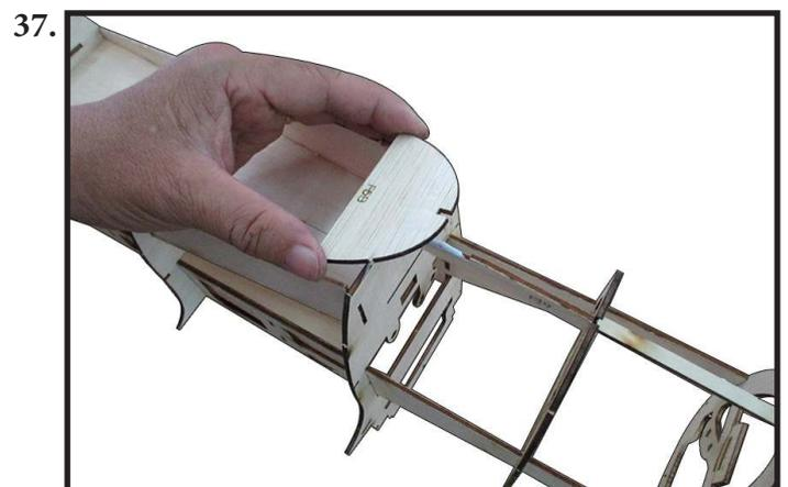
Locate and assemble F22 to fuselage by CA glue as photo shown (photo 34).
