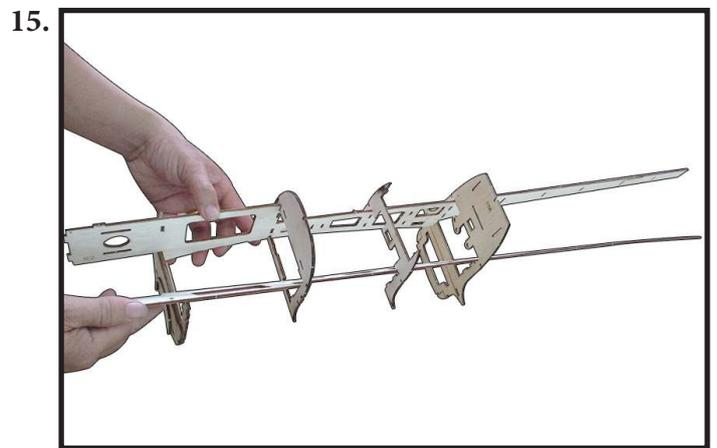
Locate and assemble FS1 to FS2 to fuselage by CA glue as photo shown (photo 16,17,18). **NOTE: The small point is regulations for the right side.**
