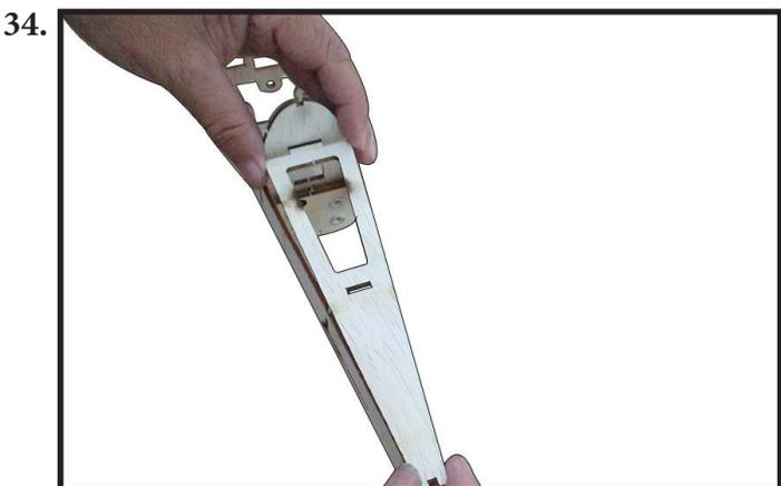
Locate and assemble H5 and F34 to fuselage by CA glue as photo shown (photo 38,39).
