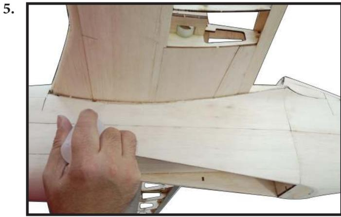
Use the paper blade cut down and use sanding tool to make flat and seamless from the fuselage to the bottom of wing (Photo 6).
