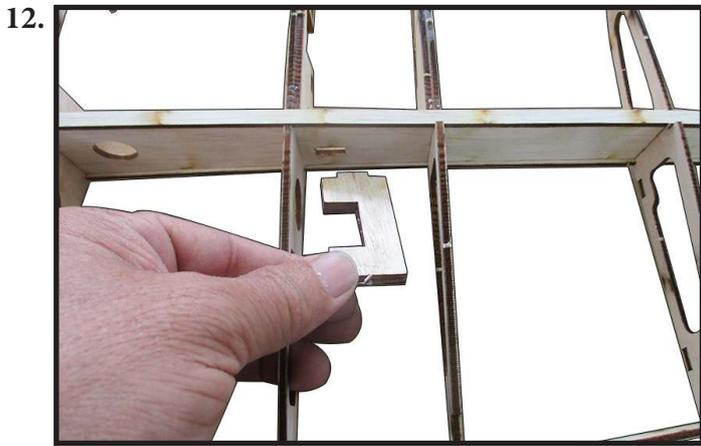
Locate and assemble gear mount (W20) by Epoxy to sure hardly as photo shown (Photo 13, 14).
