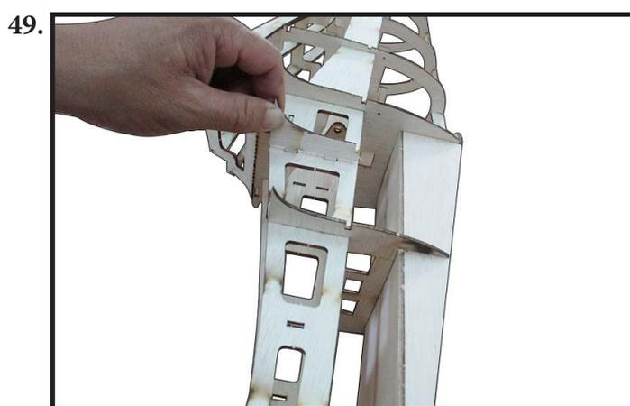
Locate and assemble F20 to right fuselage side by CA glue as photo shown (photo 50). Then, you attach F20 to the left side.
