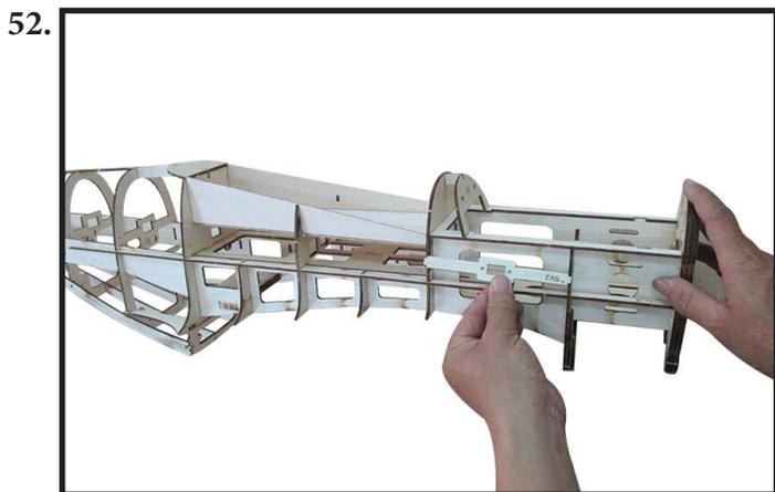
Locate and assemble SW1 to left fuselage side by CA glue as photo shown (photo 53).
