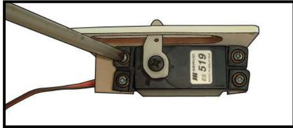
6) Apply 1-2 drops of thin C/A to each of the mounting tabs. Allow the C/A to cure without using accelerator.
