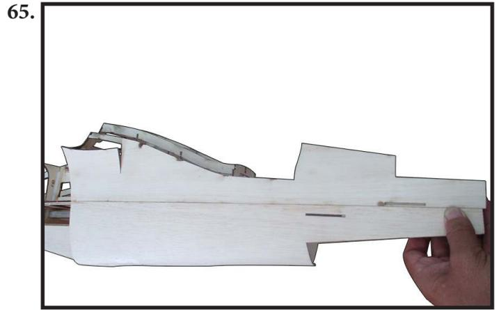
Bend the balsa sheet go to the curve of bottom area. Then, add CA glue and use the finger at this place until the glue dries as photo shown (photo 66). Do the same for the other half of the bottom area, so that the balsa sheet keep fixed fuselage.
