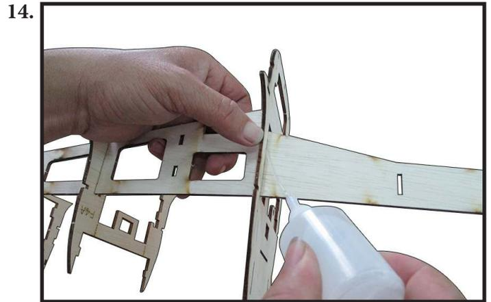
Locate and assemble left fuselage side S1 to F2 block, F3A, F4A, F5A by CA glue as photo shown (photo 15).
