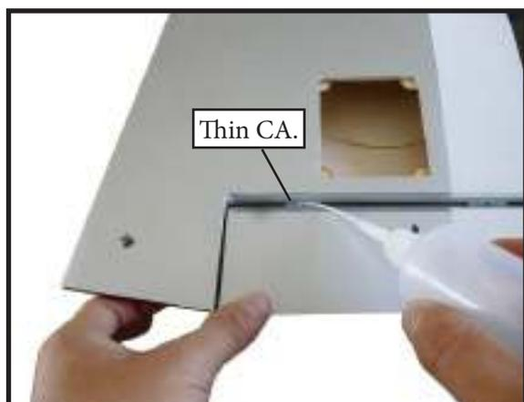
5) Turn the wing panel over and deflect the flap in the opposite direction from the opposite side. Apply thin C/A glue to each hinge, making sure that the C/A penetrates into both the flap and wing panel.
