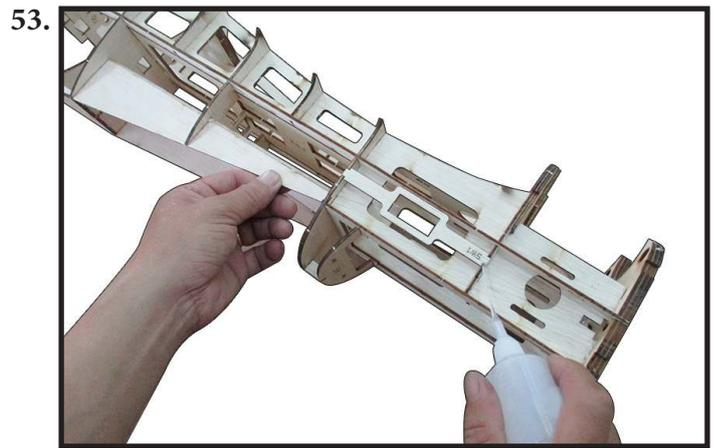
Locate and assemble F15A and F16A to right fuselage side by CA glue. Then, you attach F15B and F16B to the left side as photo shown (photo 54).
