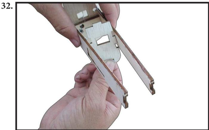
Locate and assemble F19 to fuselage by CA glue as photo shown (photo 36).
