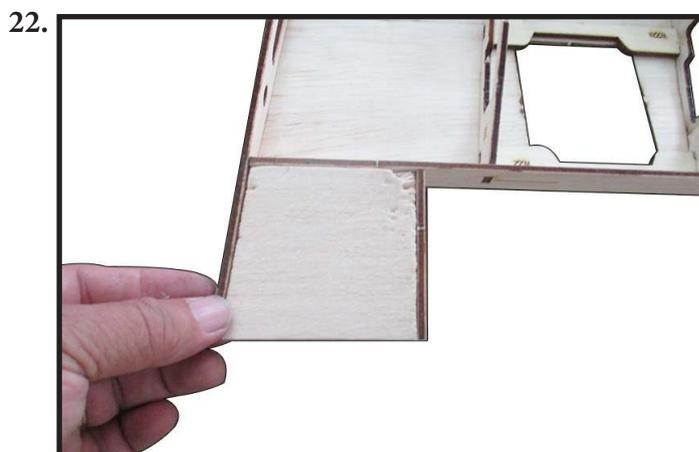
Locate and assemble W16, W17 and two hard wood bar to sure hardly by epoxy glue as photo shown (photo 23,24).
