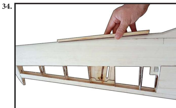
Assemble special 8mm balsa sheet W36 to wing left and wing right as photo shown (photo 35). Then, cut down W36 so that shaping as W2, use sanding tool to smooth (do like this for wing left and wing right). Join two wing panel together by wing tube (Ø 19mm). Set up two wings until they have to close touch at between (no gap) by the sanding tool. Then, locate and assemble W1 at each of wing (left and right) (Photo 36,37).
