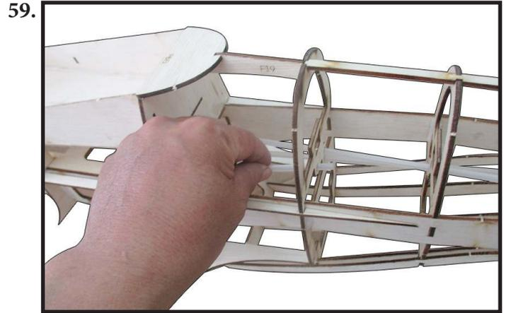
Attach the aluminum square tool bar to the square hole at each former. It is through along to fuselage to adjust to fuselage straight. Remove it after finishing covering balsa sheet for fuselage (photo 60).
