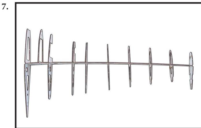
Locate and assemble W27 (Leading Edge) to front of wing, and W30 (Trailing Edge) to rear of wing as shown photo (Photo 8,9).
