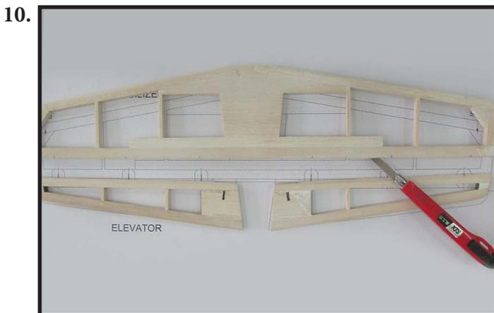
First, assemble 6 paper hinges to Stabilizer. Then, link to Elevator (Photo 11).
