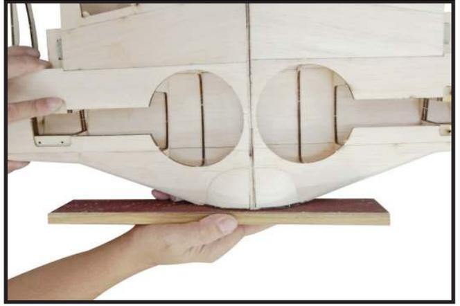
Sanding to smooth (not rough) at interface on fuselage (the edges of fuselage where the wing panel intersect to the fuselage) as photo shown (Photo 3).
