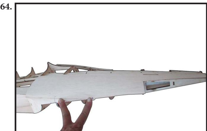
Put the sheet SH7 at bottom area and toward rear of fuselage as photo shown (photo 65).
