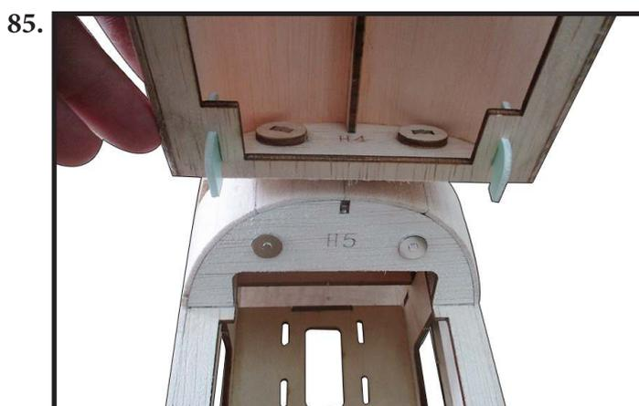
Setup the hatch and the fuselage so that the top of hatch seamless the top of fuselage by sanding tool (photo 86).
