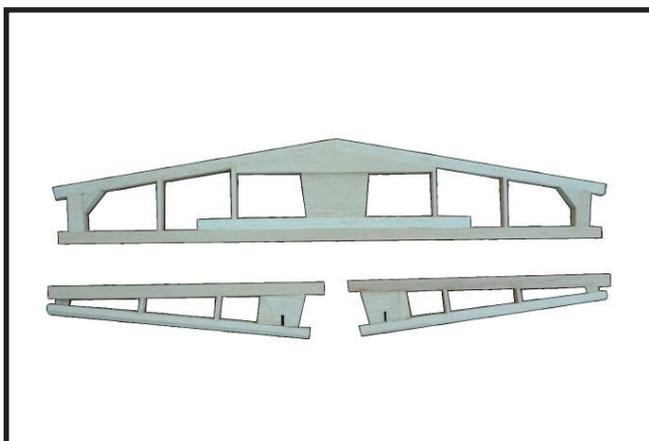
Cut off the excess balsa wood part and sanding smooth and flat the edge (Photo 5).
