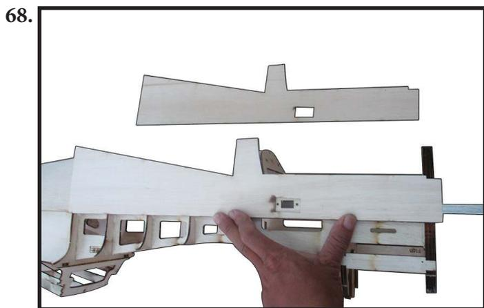
Locate and apply the sheet SH4 to fuselage ( at top ) by CA glue as photo shown (photo 69 &70).
