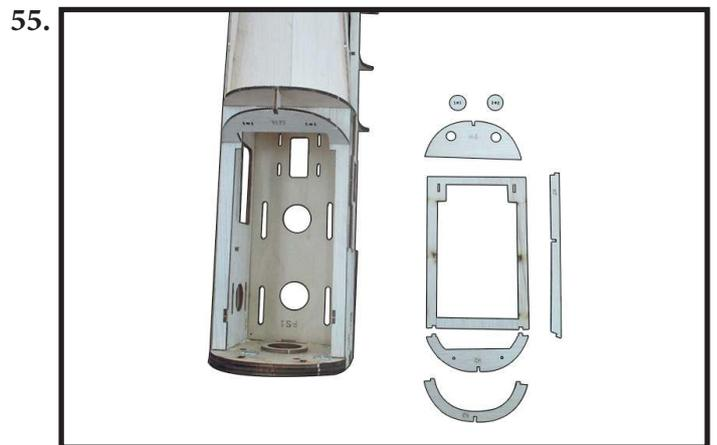
Step by step, locate and assemble H2, H3, H4 to H1 by CA glue as photo shown (photo 56).
