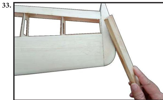
Use sanding tool to make curve shape for L.E area so that it seamless as curve of ribs, and make smooth for L.E. Note: need to keep straight (avoid rough) as photo shown (photo 34).
