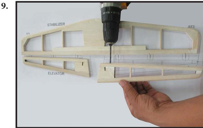
Locate position of paper hinge for Stabilizer and Elevator as plan. Then, sawn the slot ( for 6 hinges) by the blade tool (Photo 10).
