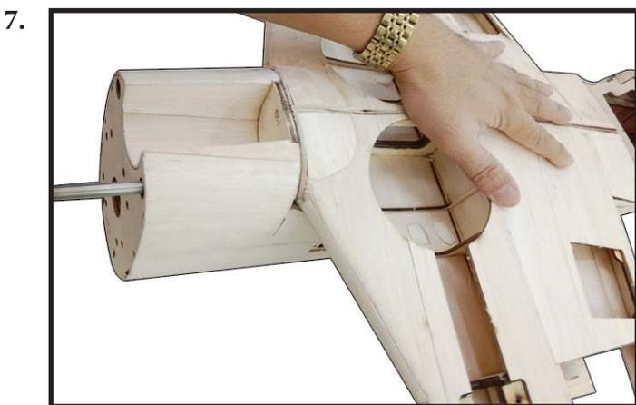
At the front of wing, drill two holes (Ø 8mm) for mounting two dowels, the center of hole is ink mark point. (Photo 8).
