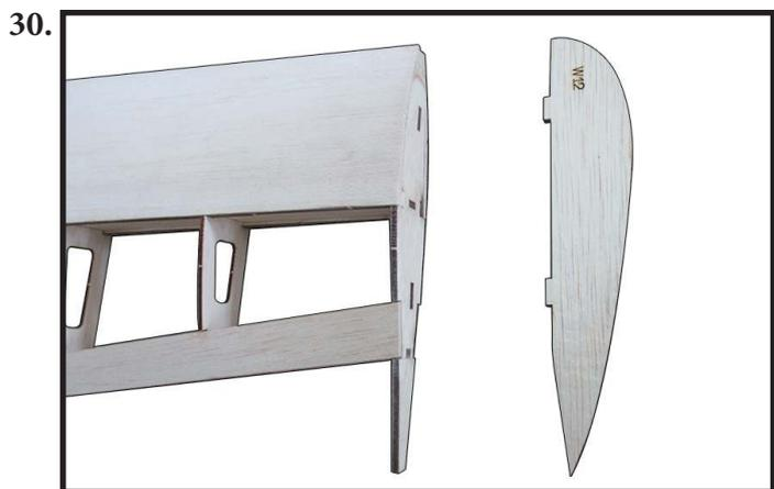
Apply two 8mm balsa sheets W13 into W12 (top and bottom) by epoxy glue. Then, cut down W13 so that shaping as wing tip, use sanding tool to smooth as photo shown (photo 31,32,33).
