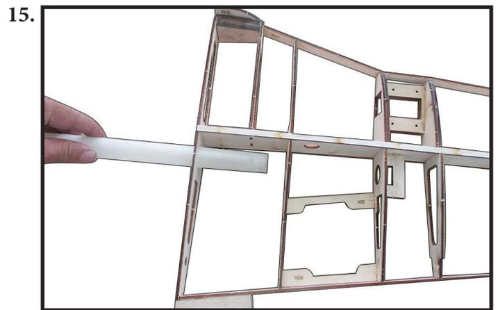
Apply the 8mm balsa block spar to W27 (Leading Edge) at front of wing, and sanding for them seamless together as shown photo (Photo 16).
