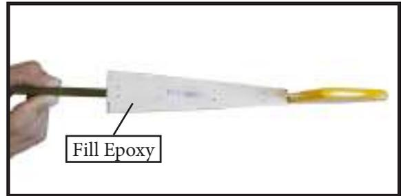
2) Slide the vertical stabilizer into the slot in the top of the fuselage. The rear edge of the stabilizer should be flush with the rear edge of the fuselage and the lower rudder hinge should engage the precut hinge slot in the lower fuselage. The bottom edge of the stabilizer should also be firmly pushed against the top of the horizontal stabilizer.
