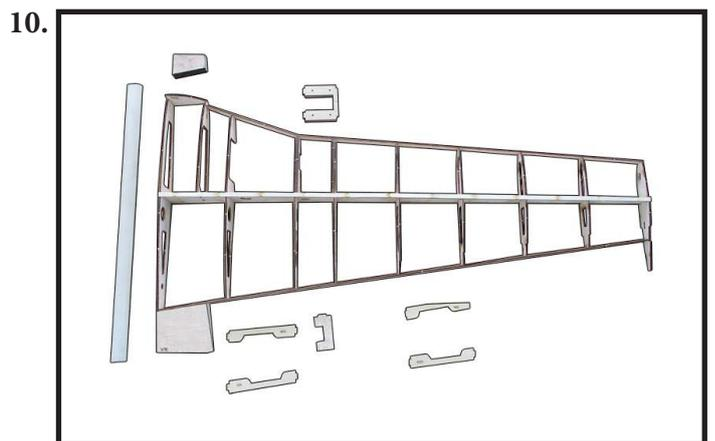
Locate and apply the balsa block (W15) to front of wing (W14) to increase the thickness at here (Photo 11).
