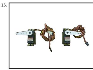
Minimum servo spec. Torque : 333.00 oz-in (23.98 kg-cm) @ 6.0V; oz-in (29.02 kg-cm) @ 7.4V
