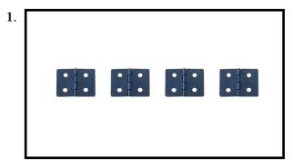
Prepare the aileron hinges by scuffing the area that will be inserted into the wing or flying surface with medium grit sand paper. Be careful not to remove too much material. Use isopropyl alchol, and a paper towel to remove any excess debris that remains on the hinges.
