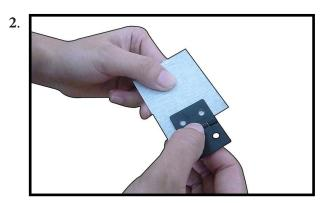
Mix a sufficient amount of 30-minute epoxy in a cup, and with a toothpick, smear epoxy in the hinge pockets of the wing panel and aileron. Slowly and carefully, insert each hinge into the wing panel. Partially remove and reinstall the hinge to ensure that you've completely coated it with glue. Clean up any excess epoxy with isopropyl alcohol, and tape the aileron in place to cure.
