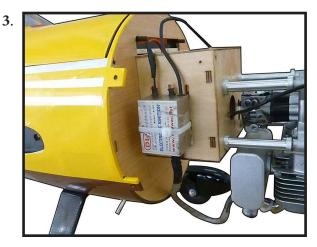
Connect ignition module to pickup line of engine. Secure with Safety Clip, safety wire, tape or other method. Ensure the plugs will not come apart from vibration or light tension. Secure ignition wire with nylon ties as necessary.
