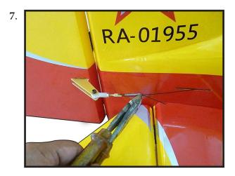
Cut off excess cable as shown.
