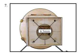
Attach the motor mount to the front of the electric motor box using four 6.5mm blind nut, four M5x25mm hex head bolts to secure the motor. Please see picture shown.
