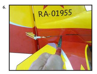
Crimp the brass tube with a crimping tool or pliers.
