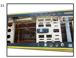
Feed one rudder cable through the pre installed cable exit tube in the rear of the fuse toward the front of the fuse. Repeat for other side.
