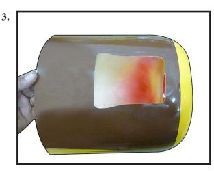
Tape the cowl to the fuselage using low-tack tape.
