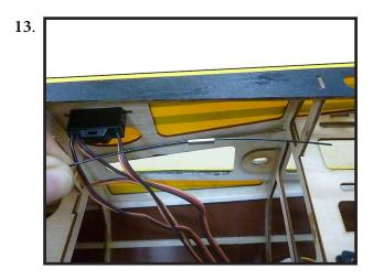
Thread cable through the threaded coupler hole, and back through the brass swage tube as shown.
