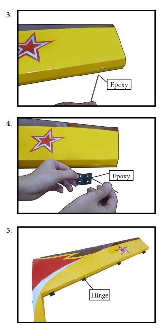
Press the aileron and wing together such that less than a 1/64" hinge line gap exists between the aileron and wing. The bevels should virtually touch. Use a paper towel and rubbing alcohol to wipe away any visible epoxy around the hinges.
