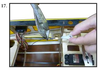
Cut off excess cable as shown.
