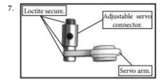
Reinstall the servo horn by sliding the connector over the pushrod wire. Center the throttle stick and trim and install the servo horn perpendicular to the servo center line.
