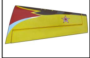
**Note** : <u>Work the aileron up and down sev</u> <u>eral times to "work in" the hinges and check</u> <u>for proper movement.</u>
