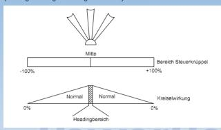
As can be seen from the diagrams above, gyro gain is suppressed progressively as control travel is increased. This reduces the effect of the **iGyro** in terms of counteracting deliberate control commands.
