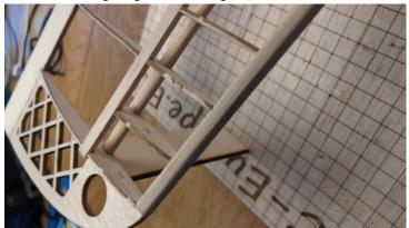
Glue the Rib1 (3mm) to the middle section and glue the tip to the middle section of the wing. With the support at the tip.
