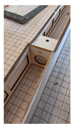
Glue in F3 and W2, W2"at bottom side to both sides
