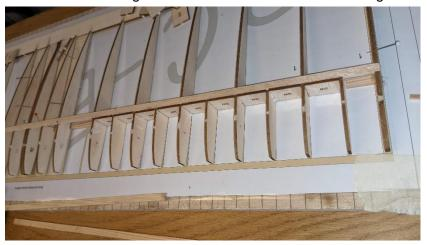
Glue in the triangle to the middle ribs and trailing edge Sand down triangles so top deck fits. Glue balsa on top of middle wing between trailing edge and spar.
