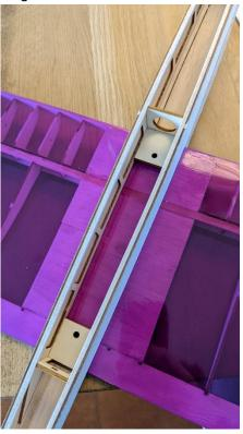
Glue the bottom side to the fuselage.
