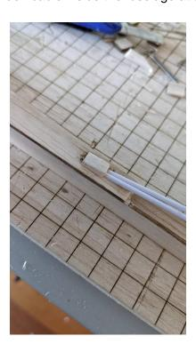
Put on the wing and mark the holes for the wing mount.
