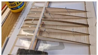
Glue ribs 1 on the spar and trailing edge.
