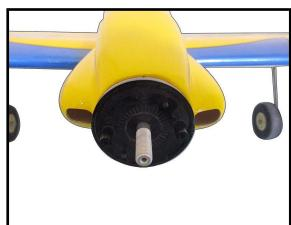
Fit the spinner cone in position. Position the spinner cone so it does not contact the propeller, Secure the spinner cone using the provided screw and 1.5mm hex wrench.
