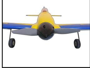
Fit the propeller on the adapter. Thread the propeller nut on the adapter and tighten the nut using a 7/8-inch socket or box end wrench.
