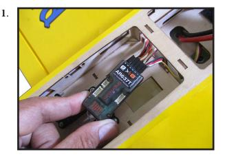
Secure the receiver in the fuselage. Use the instructions included with the receiver for additional mounting details.Make sure none of the wires from the receiver interfere with the operation of the servos.
