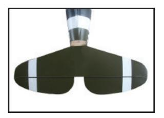
4) With the stabilizer held firmly in place, use a pen and draw lines onto the stabilizer where it and the fuselage sides meet. Do this on both the right and left sides and top and bottom of the stabilizer.
