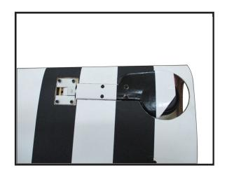
Insert bomb onto the wings.
