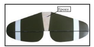
7) When you are sure that everything is aligned correctly, mix up a generous amount of 30 Minute Epoxy. Apply a thin layer to the top and bottom of the stabilizer mounting area and to the stabilizer mounting platform sides in the fuselage. Slide the stabilizer in place and realign. Double check all of your measurements once more before the epoxy cures. Hold the stabilizer in place with T-pins or masking tape and remove any excess epoxy using a paper towel and rubbing alcohol.
