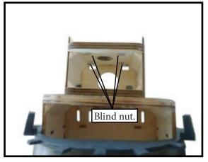
5) Attach the motor to the front of the electric motor box using four 4mm blind nut, four M3x15mm hex head bolts to secure the motor. Please see picture shown.
