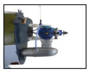
Blow through one of the lines to ensure the fuel lines have not become kinked inside the fuel tank compartment. Air should flow through easily.
