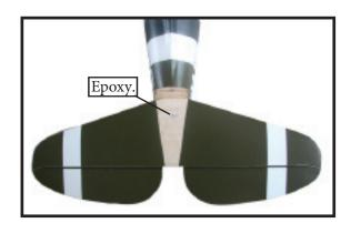
3) Slide the vertical stabilizer back inplace. Using a triangle, check to ensure that the vertical stabilizer is aligned 90° to the horizontal stabilizer.
