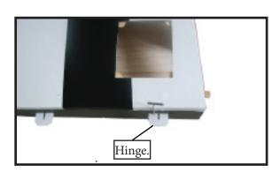
3) Slide the wing panel on the flap until there is only a slight gap. The hinge is now centered on the wing panel and flap. Remove the T-pins and snug the flap against the wing panel. A gap of 1/64" or less should be maintained between the wing panel and flap.
