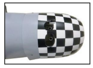
2) While keeping the back edge of the cowl flush with the marks, align the front of the cowl with the crankshaft of the engine. The front of the cowl should be positioned so the crankshaft is in **nearly** the middle of the cowl opening. Hold the cowl firmly in place using pieces of masking tape.
