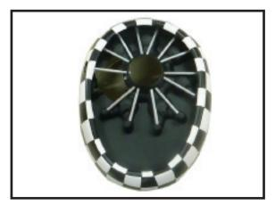
1) Slide the fiberglass cowl over the engine and line up the back edge of the cowl with the marks you made on the fuselage then trim and cut as shown.
