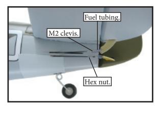
Insert fuel tank onto the wings.
