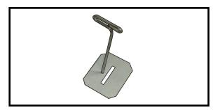
2) Remove each hinge from the wing panel and flap and place a T-pin in the center of each hinge. Slide each hinge into the wing panel until the T-pin is snug against the wing panel. This will help ensure an equal amount of hinge is on either side of the hinge line when the flap is mounted to the aileron.
