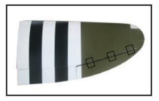
Note: Work the aileron up and down several times to "work in" the hinges and check for proper movement.
