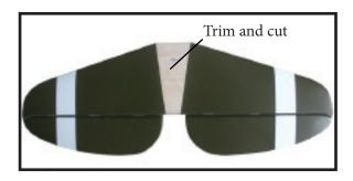
When cutting through the covering to remove it, cut with only enough pressure to only cut through the covering itself. Cutting into the balsa structure may weaken it.
