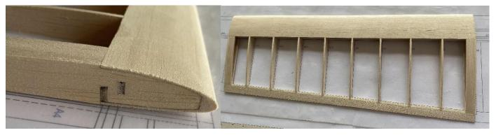
8) Assemble the wing tip&rib and wing plate, and glue the wing trailing edge.
