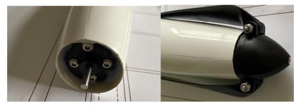
2) Position the hole with the template, install the tee nuts on B24 plywood inside of the fuselage, and fix to the body with epoxy glue. (Starch or other substances can be added to the resin glue to reduce the fluidity of the glue.)
