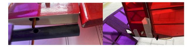
6) Glue servo mount, install the servo, and connect the rudder with the pull-pull rope.
