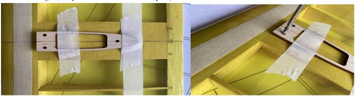
14) Assemble 6 pcs of B1 balsa and insert 5MM carbon tube, keep the carbon tube in the middle position, then assemble both wing ribs, and glue 1MM carbon sheet at the rear edge.
