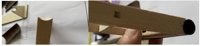
19) Glue 1MM plywood on the right side of the vertical tail, and fix the servo with double-sided tape or other glue (adjust the neutral point of the servo before fixing the steering gear). Servo wires are threaded through the hole at the bottom, then glue 1MM plywood on the left. The servo will be removed.
