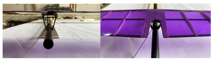
5) Compare the position of the servo wires, and drill a 4MM hole in the tail tube, then thread the servo wires into the tail tube. Connect the servo extension wires to the position of the cabin, glue the vertical tail and the carbon tube, and pay attention to adjusting the verticality.
