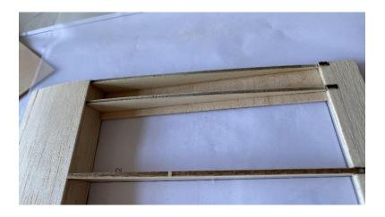
4) Glue 3 pieces of A36 into one piece and fill them into the middle of the A1 wing rib with wood glue, and glue upper covering.(3pcs of A36 are used as reinforcement for fixing screws later)
