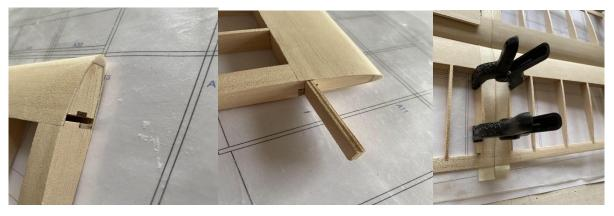
13) After joint the left and right wings, use the template to position and drill the fixed holes. (The left and right wings are fixed without glue, easy to disassemble and transport).
