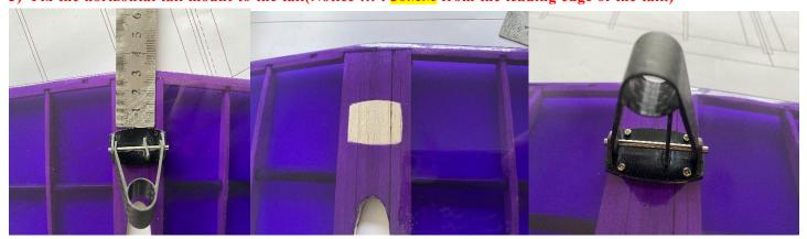
4) Glue the mount to the tail with epoxy glue, and keeping it level.
