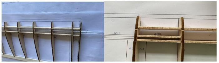
2) Glue the upper and lower wing coverings, and glue 8X12MM balsa strips to the leading edge of the wing and polish it.
