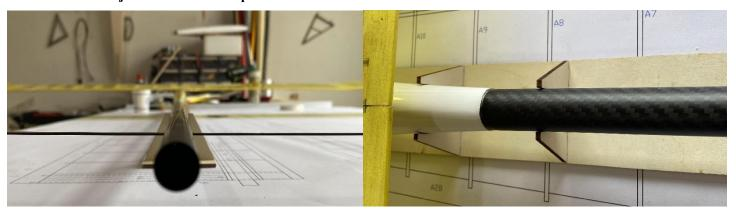
2) Assemble the horizontal tail mount and fix it with glue.
