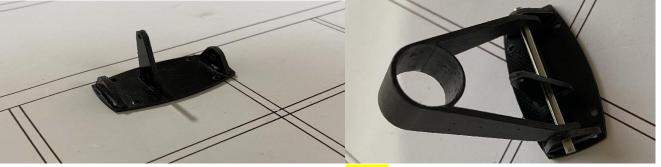
3) Fix the horizontal tail mount to the tail(Notice !!! : 30MM from the leading edge of the tail.)
