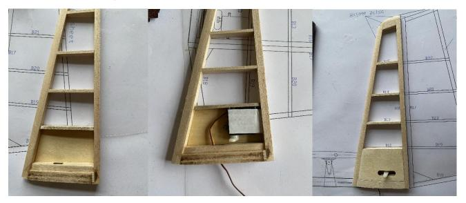
20) Assemble the rudder according to the drawing and polish the V-shaped angle.
