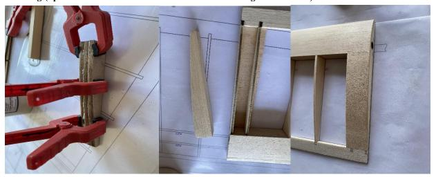
5) Cut 3MM balsa pieces into 10MM width and glue to the wing ribs for strengthening.
