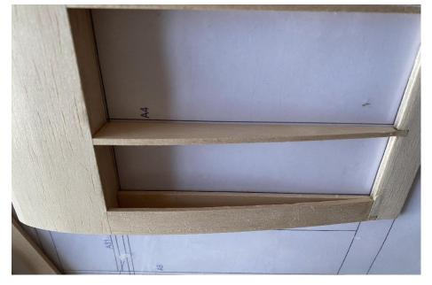
6) Assemble the middle wing rib and wing plate, and glue the wing trailing edge.
