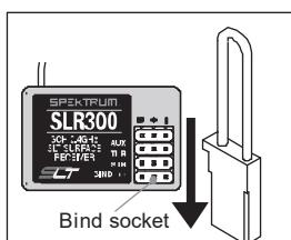
Insert the Bind Plug in the BIND port on the receiver.
