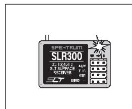
The receiver LED will stop flashing.
