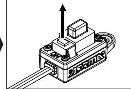
3. To enter the selected variable, release the set button on the desired number of flashes/beeps.
