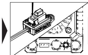
4. Using the tuning chart, press the 'set' button until the number of red LED flashes and short beeps equals the required value.
