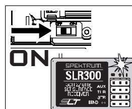
Power on the ESC. The red LED flashes, indicating the receiver is in bind mode.
