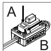
4. Switch off ESC to complete setup
