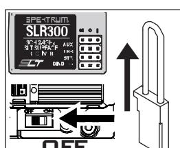
Remove the Bind Plug, then power off the ESC to save the settings.
