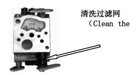
NOTICE: The carburetor fuel screen should be cleaned periodically also. Carefully remove the pump cover (inlet side of the carburetor), gasket and pump membrane. The screen will be visible and can be cleaned after careful removal.
