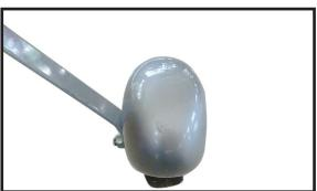
Repeat steps to install remaining wheel pants to the landing gear.
