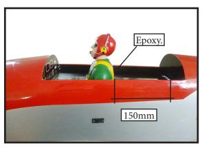
4) Position the canopy onto the fuselage. Trace around the canopy and onto the fu¬selage using a felt-tipped pen. Carefully cut and remove covering material from the fusealge where the canopy makes contact, exposing the bare wood. The permanently glue the canopy in place with epoxy glue or special "canopy glue".
