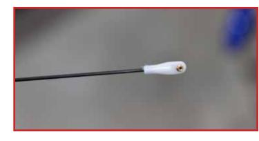
Assemble the throtle pushrod connector onto the throttle servo arm so that it can spin freely. Add a drop of CA to the nut to lock it in place so it doesn't vibrate off.
