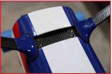
Locate the carbon fiber landing gear. Note that it has a front and a rear, it is designed to sweep forward toward the nose of the airplane. Locate the Main Landing gear hardware pack.
