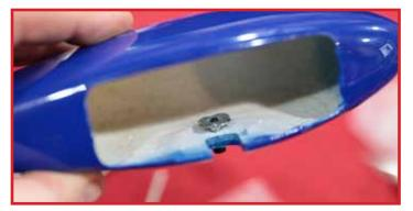
Install the wheel pants onto the landing gear. Apply loctite to the 3mm screws and fully install them into the blind nuts and tighten as shown.
