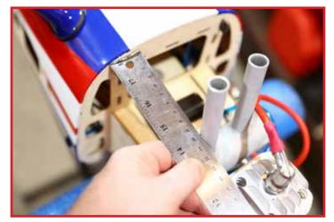
Working slowly, checking fit often, enlarge the openings until the cowl slides smoothly on and everything has clearance. Note that we have shown the minimum amount of opening, which is fine for cool weather. During the hot Summer, your engine may need more cooling air
