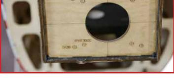
Drill the firewall for the power system of your choice. Start with a 1/8" (3mm) drill bit and expland the holes with a larger bit of the correct size for your mount screws.
