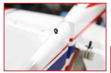
Locate one of the small ball-link ends, and using CA glue, install it into the hole you drilled in the rudder, as shown. This will be the guide for the tiller-wire which steers the tail wheel.
