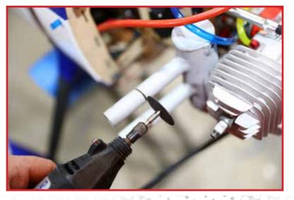
For this installation of a J&A pitts muffler, we trimmed slightly more than one inch (25mm) from the length of the outlet tubes to allow the cowl to slip over.
