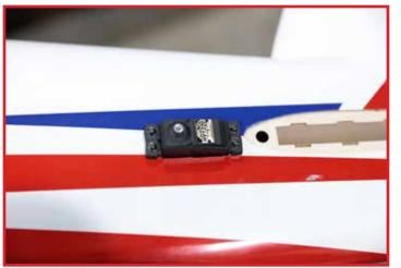
Attach a servo wire extension onto your elevator servo and secure it with a connector lock or tape. We recommend a 24" (60 cm) extension for the elevator servo. Install the servo into the fuselage. We recommend Extreme Flight RC socket head servo screws.
