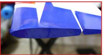
The holes in the wingtip match up to these holes in the SFG's and wingtips.
