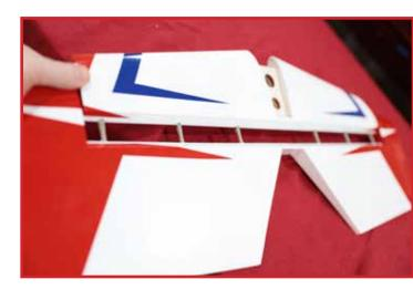
Once you have the parts fit together, make sure the elevator can flex up and down at least 45 degrees. There should be a small gap, about 1/32'' (1mm) between the stabilizer and elevators. Allow the epoxy to cure.
