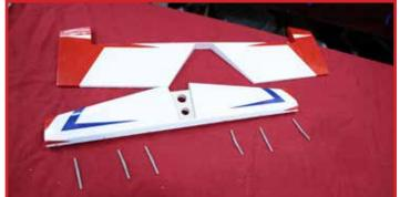
First, we must protect the hinges from any glue entering the moving portion. Place a drop of lubricating oil into the center portion of the hinge where the axle pin is. It only takes a tiny amount of oil. If you accidentally get oil on the gluing portion of the hinges, clean it off with alcohol.
