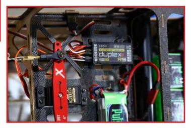
For electric power, use strong velcro straps to restrain the lipo battery packs as shown.
