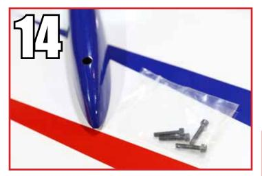
The wingtips of your Slick have 3mm nuts installed to attach the wingtips/SFG's. Open the covering as shown to expose the nuts.
