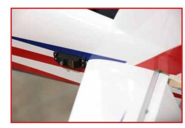
Locate the balsa block you previously removed from the tail. Slide it into position. Make certain the elevator swings freely without interference from the block. The block is soft balsa, it can easily be trimmed or sanded to correct any interference. Once you are satisfied with its fit, glue it in place with epoxy or CA glue.
