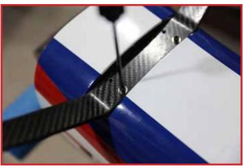
The landing gear-to-fuselage fairings are attached to the landing gear and fuselage with Shoe-Goo type silicone adhesive. First, slide the fairings onto the gear, and check for fit to determine the front and rear.
