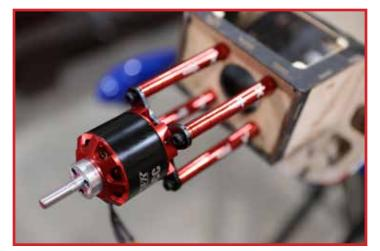
The bottom of the motor box on your Slick is design witha custom mounting area for Castle Creations Edge 80HV and 120HV speed controllers. The speed controllers mount using 4 servo screws.
