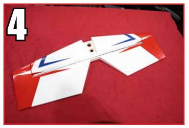
Pull the elevators and stab apart and remove the six hinges.
