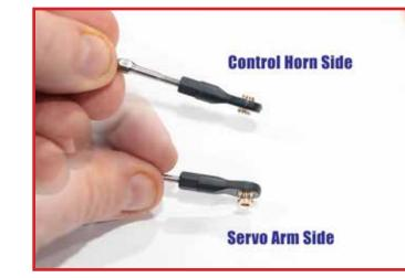
Assemble the elevator control horn as shown, using a 3mm screw with integral washer, ball link, washer and nyloc nut.
