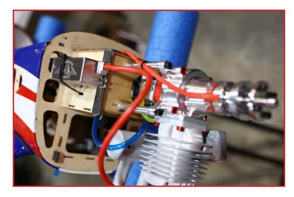
We recommend an Extreme Flight RC Flowmaster 17 oz. fuel tank. Place vibration-absorbing foam between the fuel tank and tray, and restrain the tank with velcro straps. Use Extreme Flight RC fuel tubing to make your plumbing connections. Make a loop in the overflow vent as shown.
