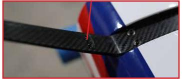
Place a large dollop of goo-adhesive onto the gear leg as shown, then slide the fairings into the gear legs. The Goo will fill up the end of the fairings. Place an additional dollop of Goo where the fairings contact the fuselage. Allow the Goo to dry while you install the wheels and wheel pants.
