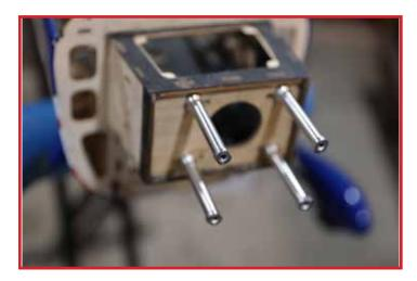
Install the standoffs which came with your DA engine using loctite.
