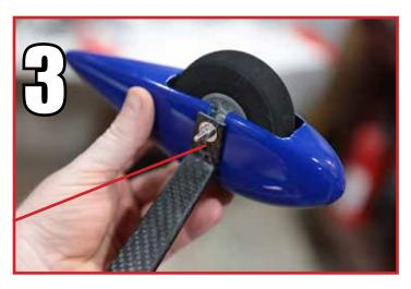
Drill the wheel pant on the mark you made as shown. Start with a 1/8'' (3mm) bit.
