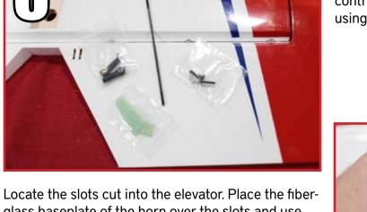
glass baseplate of the horn over the slots and use it as a template to cut the covering to expose bare wood.
