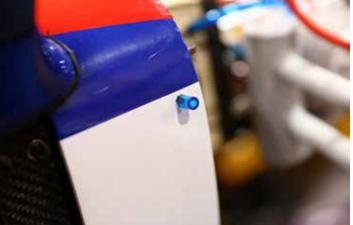
Measure the location of the exhaust outlets from the firewall. Transfer this dimension to the bottom of the cowl and cut the required openings. We use a Dremel tool for this job - protect your eyes and lungs from dust.
