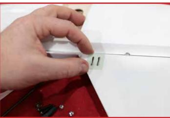
If necessary, clean out the slots in the elevator of any stray wood fibers so the control horn can easily be inserted.
