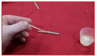
Increase the drill size until you can press the blind nut into the hole as shown. Use the 3mm screw and washer to draw the blind nut into the hole part way and the spikes on the blind nut engage the fiberglass.
