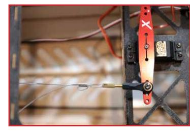
Note that while we need our rudder cables to be snug, and not slack or droppy, we also do not want them overly tight. We adjust our cables with the servo and the rudder at center to be *just snug*. Too tight cables put additional strain on the rudder servo. Also, it is normal for the cables to have some slack on one side at full deflection.
