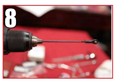
Install the servo arm and pushrod. We recommend Extreme Flight RC aluminum servo arms. Pictured is a 1.5" arm, but we recommend a 2.0" arm for maximum options in control throw. Install the pushrod with 3mm hanrdware, note that you must use either a nyloc nut or loctite on the screw which attaches the ball link to the servo arm.
