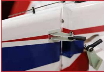
Locate the elevator pushrod, and remove the balllink from the elevator horn. To assemble the elevator pushrod, you will need to screw the ball links onto the elevator pushrod. We prefer to use a cordless drill. Chuck the bare pushrod in and hold the first ball link, and screw in as shown. Then, we turn the shaft around, and chuck the ball link into the drill to install the second ball link. NOTE: both ends of the elevator pushod are conventional "right hand" threads.
