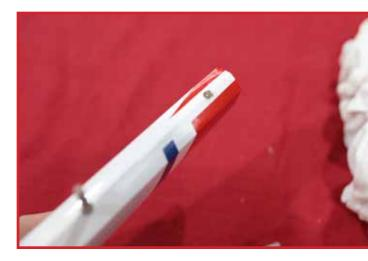
When you press the hinges into the hinge holes, some epoxy may squeeze out. Use alcohol on a rag to clean up any excess epoxy.
