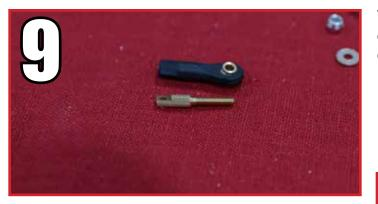
The rudder connnection is by pull-pull cable. The ends of the cables are made by screwing the brass cable ends into the nylon ball links.
