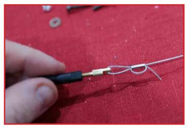
Locate the openings in the rear of the aircraft for the cables, and thread the cable inside. Install the contorl horn end of the cable onto the horn with 3mm screw, washer, and nyloc nut. thread the other end of the cable inside the fuselage to the front.
