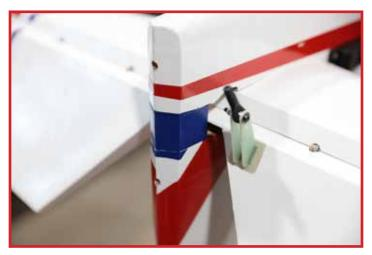
Locate the rudder and rudder hardware pack. the rudder hinges will be installed into the fuselage and rudder using the exact same technique you employed to install the elevator hinges in step 4. Once the rudder is installed, allow the epoxy to cure.
