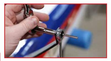
Slide wheel collars onto the axles, then the main wheels, then outer wheel collars. The wheel collars locate the wheels on the axles, when you install the pants you will need to fine-tune the location of the wheels. Apply a drop of loctite to the set screws in the wheel collars and tighten them.
