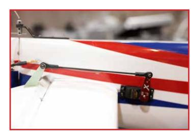
The rudder horn is double-sided. Use sandpaper or an emery board to scuff the middle part which will Igue into the rudder. Assemble one side with ball link as you did the elevator horn. Place part-way into the rudder and shown
