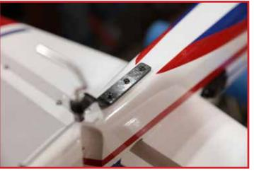
Install the two tail-wheel collars and the tail wheel as shown. Use Loctite on the set screws of the collars.
