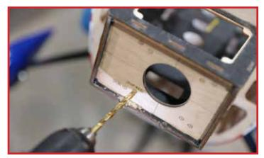
For XPWR 30CC electric power, install the bases of the Extreme Flight STANDARD-LONG Blazing Star standoffs with loctite. Install the extensions to achieve 95mm length, then install the motor using loctite. For any installation, the distance between the firewall and spinner backplate is 163mm.
