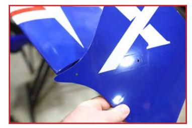
Screw on the wingtips and SFG's on as shown. Because these parts need to be removed for transporting the aircraft, do not loctite these screws. Locate the hardware for the wingtips and Side-Force generators (SFG's). Installing the wingtips and/or SFG's is purely optional. SFG's increase stability in 3D flight and increase rudder authority. We recommend you try all combinations to determine which you like best.
