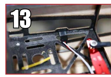
Mount your receiver, and tie all wires to prevent vibration damage.
