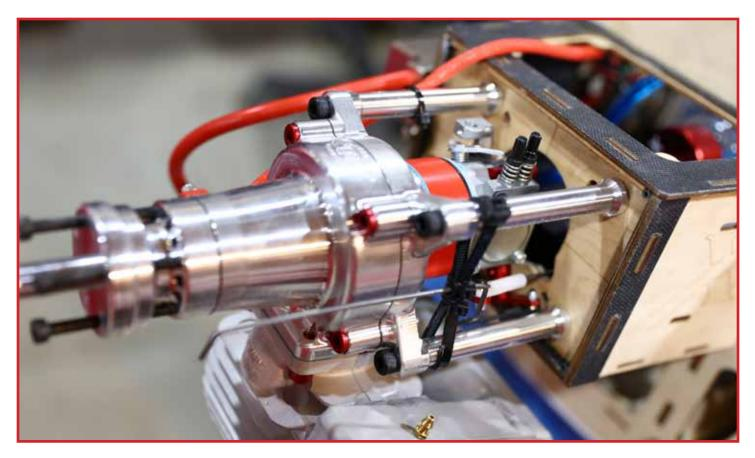
Ther are a variety of choke linkages possible on the DA-35. Here, we illustrate a forward choke, accessed through the cooling hole on the front of the cowling. We use zip ties as shown to make a bracket for the rod to slide through. The choke arm on the carburetor may need to be loosened and rotated for the choke linkage to work optimally.
