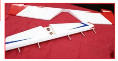
Put several large drops of epoxy in the hinge holes in the elevator and fit the elevator and stabilizer together. Clean up any excess epoxy which squeezes out.
