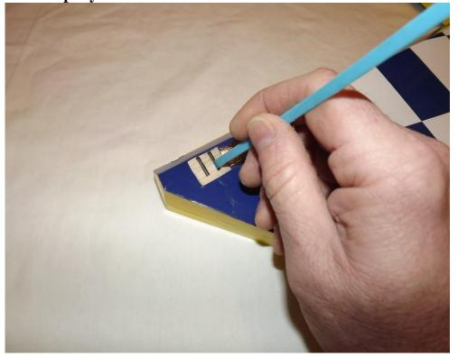
7. Apply a generous amount of epoxy to the bottom of the G-10 control horns and base plate.
