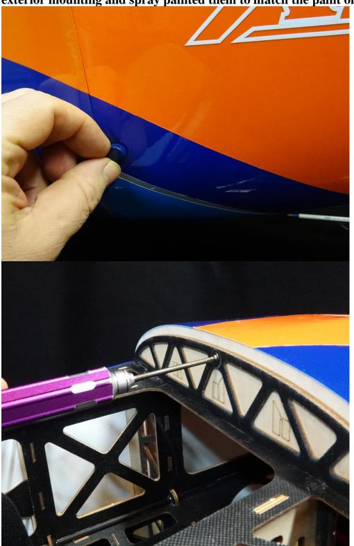
36. Attach a 36 inch EF 20 awg servo extension to each elevator servo lead. If you plan to remove the stabs for transport, you will need to use 48 inch extensions. Secure with EF Servo Safety Clips or heat shrink tubing. Slide the stab halves onto the carbon fiber stab tube and secure with a 3mm bolt and washer inserted through the mounting tabs and into the pre-mounted blind nuts. Make sure to use a drop of blue Loctite on these bolts.
