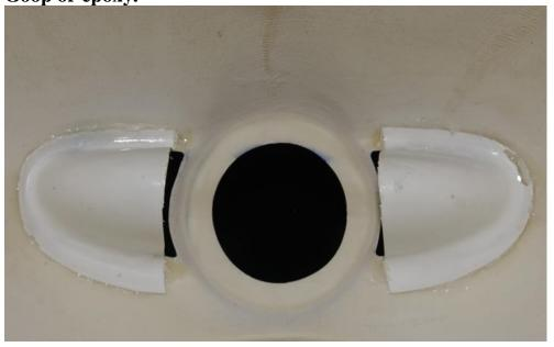
35. The cowl has a unique method of mounting that allows easy installation and removal. It is secured with 3 3mm bolts, 2 on the lower external portion of the cowl and one mounted from the interior of the fuselage. The cowl hangs on 2 hooks and is secured at these 3 locations. I chose to use 2 of the EF Thumb Screws for the exterior mounting and spray painted them to match the paint on the cowl.
