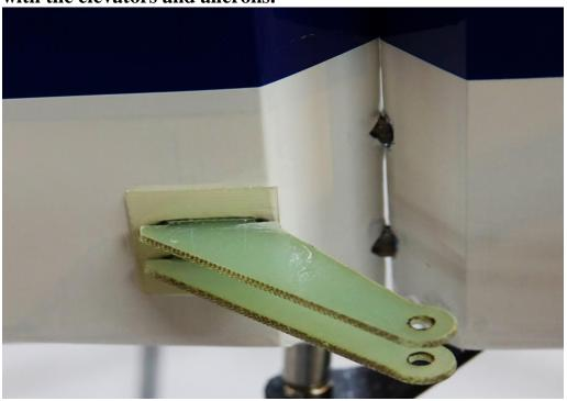
28. As mentioned there are two locations available to install the rudder control horns. If using the pull-pull system use the upper horn location as shown in this photo.
