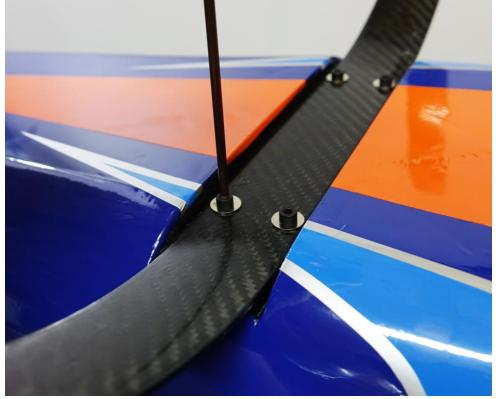
19. Trail fit the landing gear fairings and when satisfied with fit secure with Goop
