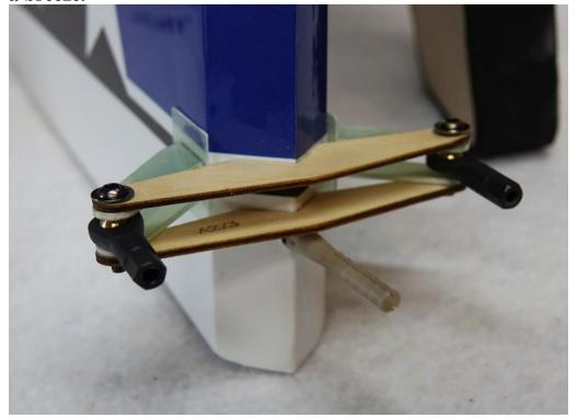
29. Once your control horn installation has cured, mount the rudder to the fuselage using the same process as you did when gluing on the ailerons and elevators.
