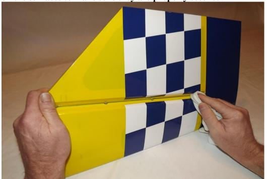
Note: Before installing the servos, it's a good time to seal the hinge gap with a strip of Ultracote or Blenderm tape. Also, I recommend that you dilute a small amount of epoxy with a few drops of alcohol and apply a light coat to the inside of the stab and to the servo mounting rib as well as to the root rib and mounting tabs to protect against exhaust residue that can collect in these areas, especially if you plan to run a smoke system.
