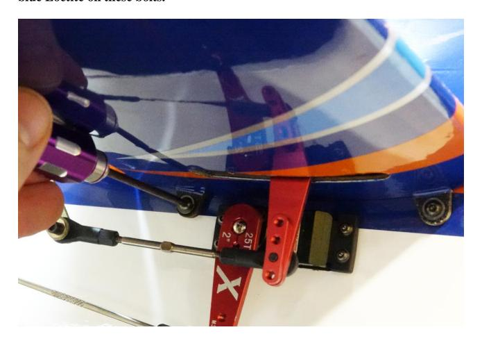
37. The wings are mounted on the provided carbon fiber wing tube and retained by inserting a 3mm bolt and washer through the two tabs that protrude from each wing root and into the corresponding blind nuts that are mounted in the fuselage structure. Be careful not to cross thread the bolts. Also, included with your Extra 330E is a set of side force generators (SFGs) and racing tips. They are secured to each wingtip with 3mm bolts inserted into pre-installed blind nuts in each wing tip.
