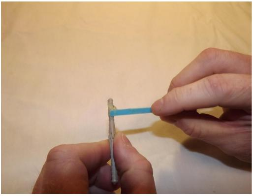
11. Make sure the hinge pins are centered in the hinge gap and that they pivot 90 degrees to the stab.
