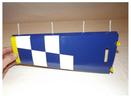
12. Now coat the other side of the hinges as well as the hinge holes in the elevator with epoxy and install the elevator onto the stab. Don't forget to apply epoxy in the hinge holes on the stab before installing the stab to the elevator.
