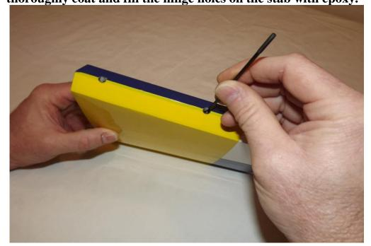
10. Next, coat one side of the hinges with epoxy and push the hinges into the holes of the horizontal stab.
