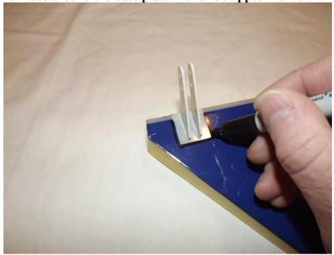
3. Remove the horn assembly and use a #11 blade to remove the covering from inside the ink line you traced around the control horn base.
