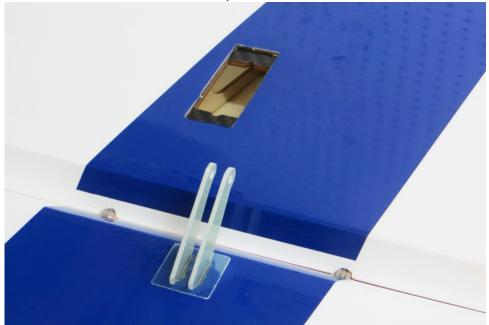
17. Attach a 12 inch EF 20 awg servo extension to the aileron servo lead and secure with a servo safety clip or heat shrink tubing. Install the aileron servo using the manufacturer provided hardware with the output shaft oriented toward the leading edge of the wing. Electronically center your servo and install the 1.5" EF servo arm and linkage as shown.
