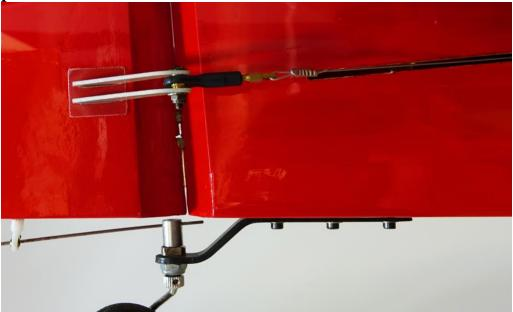
There is a plywood jig included in the hardware package to help properly align the dual control horns if using a pull-pull setup. This makes achieving correct alignment a breeze.
