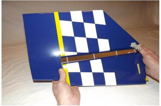
13. Use denatured alcohol and a cloth to remove all excess epoxy, especially on the hinge pin. Make sure you have full deflection in both directions — once satisfied with the results, set the surface aside to dry. After the hinges have dried thoroughly, pull on the surfaces to make sure they are properly secured.
