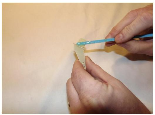
8. Reinsert the assembly into the elevator and wipe away any excess epoxy with a cloth and denatured alcohol. Place a 3mm bolt through the horns to help insure proper alignment and set aside to dry. Repeat for the other elevator half.
