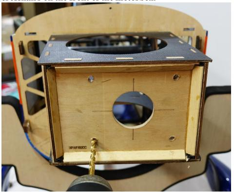
24. We highly recommend using the Blazing Star XXL Standoff Set to easily and accurately mount your Xpwr motor to the Extra airframe. All necessary mounting
