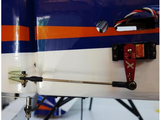
32. If using a pull-pull setup now is the time to install the pull-pull rudder cables. Install the cable onto the brass threaded connector as shown, using the aluminum arises tube to secure
