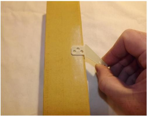
6. Apply 30 minute epoxy to the elevator slots using a zip tie to ensure the slots are filled will epoxy.
