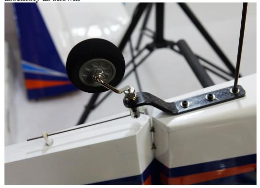
31. Attach a 36" EF 20awg servo extension to your rudder servo and secure with an EF Servo Safety Clip. Install the rudder servo in the rear of the fuselage as shown if using a direct drive rudder actuation setup and assemble the linkage as shown with
