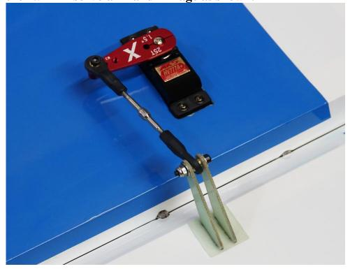
Note: Before moving to the next step – it would be a good time to seal the hinge gaps with a strip of Ultracote or Blenderm tape. Be sure to fully deflect the control surface when sealing the gap to allow for full deflection once the gap is sealed.
