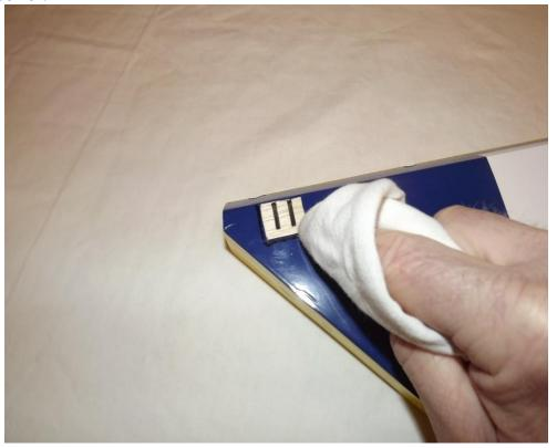
5. Use sandpaper to scuff the portion of the horns and base plate that will be inserted into the elevator.
