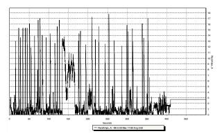
In the example above, the average current was 2.62 amps, which calculates to 435mAh per 10 minutes (typical flight length). It's recommended that only 60% of the available capacity be used to ensure plenty of reserve battery capacity. In this example, using two 4000mAh batteries (8000mAh total capacity) x 60%= 4800mAh (available usable capacity) divided by the capacity used per 10-minute flight. 435mAh would allow up to 11 flights of 10 minutes each.
