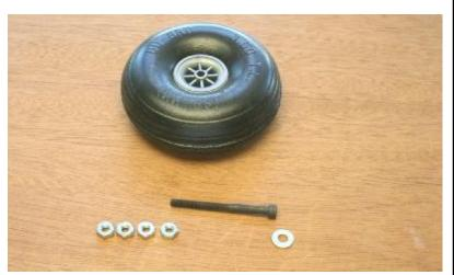
2...Place a washer on the axle screws. Insert the axle screws into the wheels. Install one nut on the axle and screw it down to the wheel. Back the nut off 1 turn to allow about 1/32" side play in the wheel. Now install a second nut to lock the first one in place. Now install a third and fourth nut as a spacer. Use a thread locking compound on these nuts.
