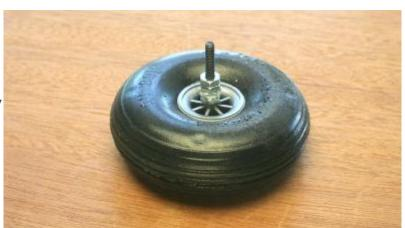
3...Insert the axle into the landing gear and secure with a nut. Use a thread locking compound on this nut.
