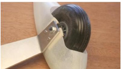
11...Repeat to install the wheel pant on the opposite side. Make sure the wheel pants are aligned with each other.
