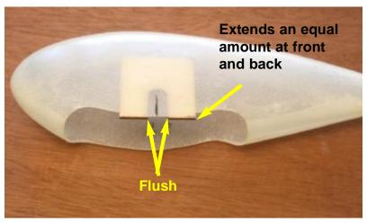
6...Using the slot in part LG as a guide, cut away the fiberglass with a Dremel tool or a file. Trim or sand the bottom edge of LG flush with the edge of the wheel pant.
