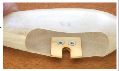
10...Install the wheel pant to the gear leg with two 4-40 x 3/8" screws. Check to make sure that the wheel rotates freely. Cut off the excess from the axle screw as shown.
