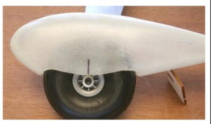
5...Place part LG on the inside of the wheel pant as shown. The inboard corners on the bottom should be flush with the wheel pant. The outboard corners of LG should extend below the edge of the wheel pant an equal amount. Glue part LG to the inside of the wheel pant with thick C/A glue.
