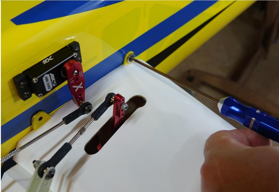
**17. Slide the wing tube into the fuselage socket and slide the wings onto the tube. Connect the aileron servo extensions to the receiver (this is where the EF mutli-plug is of great benefit, please see picture).**
