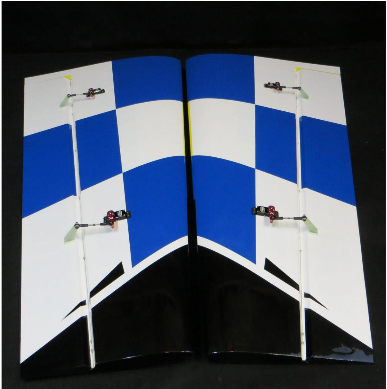
**4. Install the elevator servos, orient the output shaft toward the hinge line of the horizontal stabilizer. It will be easier to install the servo arms after mounting the servo. Make all hookups for the pushrods/ball links as we did in the previous step. I recommend using the 1.75" location on the 2 inch servo arm to maximize mechanical advantage and minimize the chance of flutter.**
