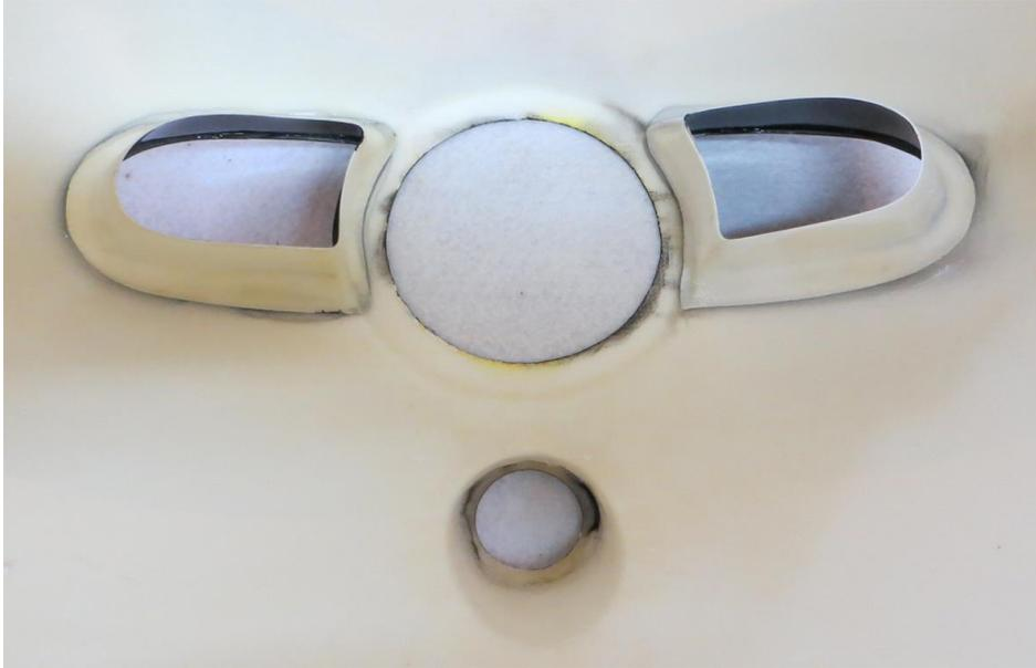
**14. Mount the cowl using the 3 3mm socket head cap screws and washers. The longest of the 3 bolts is used to secure the bottom of the cowl and the remaining bolts secure the top of the cowl as shown. Be sure to use blue Loctite on these bolts.**
