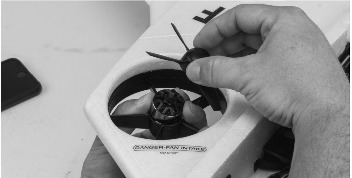
4. The rear motors use a traditional fan nut and spinner but do have different thread directions as with the front motors. Place the propeller over the appropriate motor, paying close attention to the direction (reference the diagram on the previous page). Place a fan washer over the fan on the motor shaft, followed by the fan nut. Tighten the nuts completely with an adjustable wrench.
