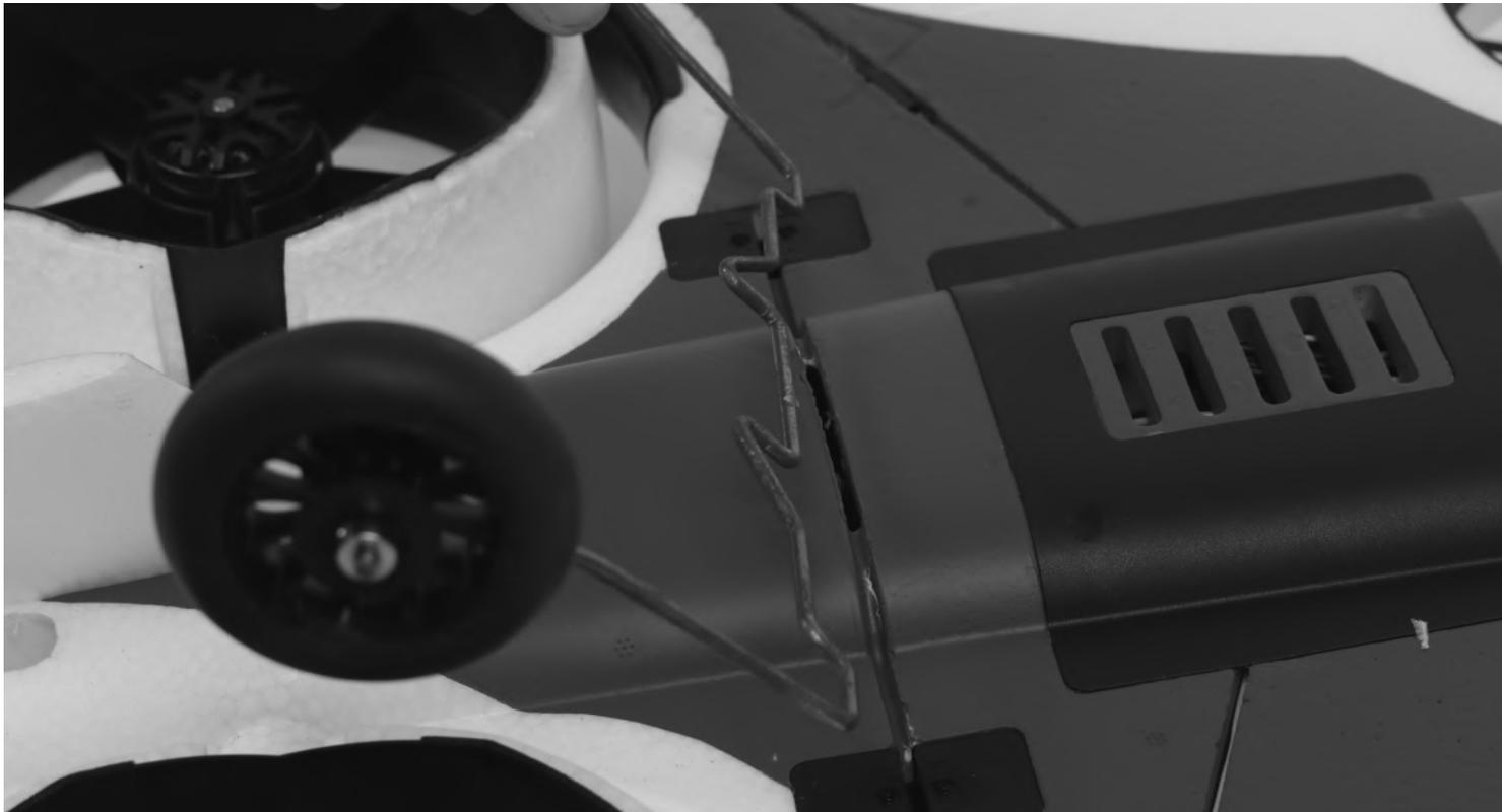
2. Place the retaining plates over the landing gear wire in the slot in the fuselage, noting that their orientation matches the landing gear wire shape. Secure them in place with two M3x8 self-tapping screws. Do not over tighten.
