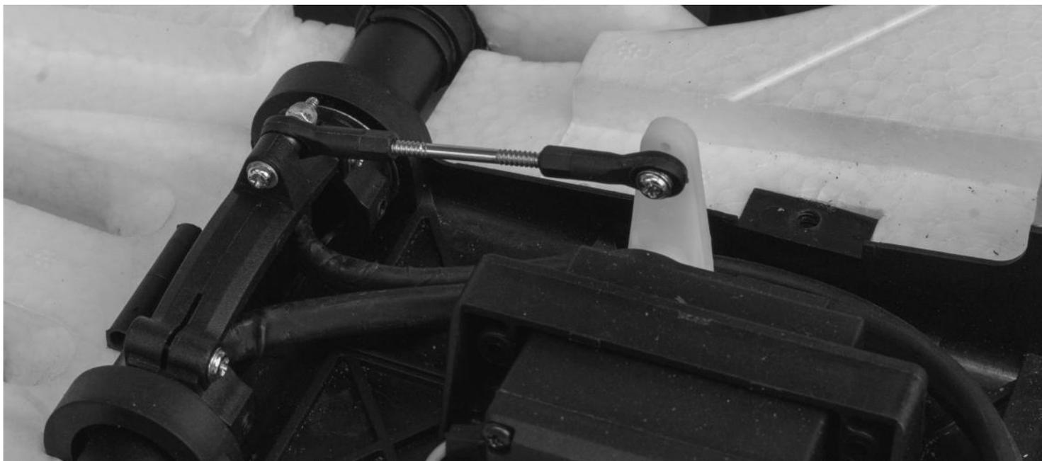
2. Move your Flight Configuration switch (channel 6) to the 45 degree "Magic Mode" position. Align the provided 45 degree gauge with the panel line on the top surface of the wing and the center of a rear fan. Adjust the tilt angle by shortening or lengthening the linkage. Set the angle of the rear fans so that they match the provided gauge.
