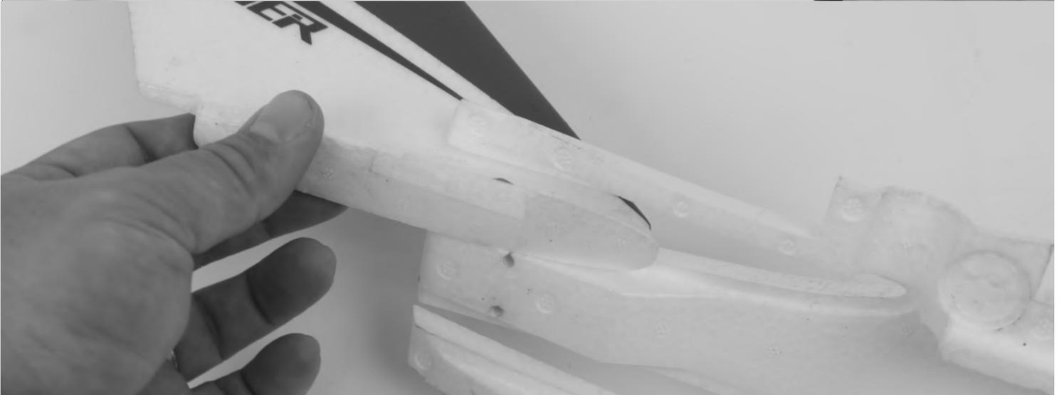
2. Once the vertical fins have dried, use a #1 Phillips screwdriver and the screws removed in the tilt setup section to secure the rear hatch assembly onto the fuselage. Note that the two shorter screws are used for the rear mount locations, and the longer screws are used for the front mount locations.
