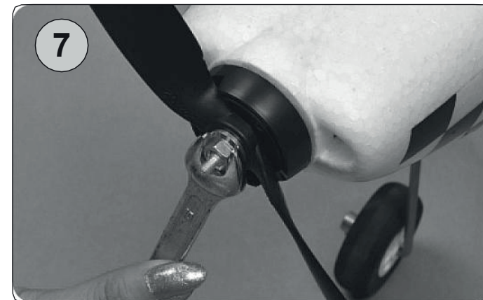
Picture 3 - 7 Put the prop hub onto the motor shaft. Then mount the spinner backplate, the prop, washer and nut. Tighten the nut carefully but firmly to avoid it gets loose in flight.
