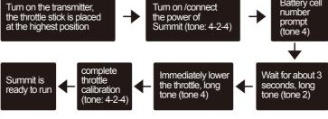
. If R/C throttle signal is reversed, the ESC may enter the calibration incorrectly Please pay special attention to this, power off, reverse the throttle signal and try again.
