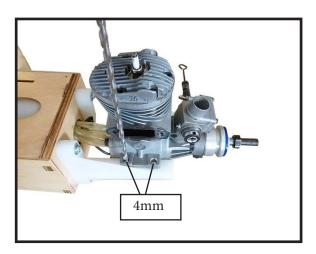
3) Use a drill to drill the four holes in the engine mount rails.
