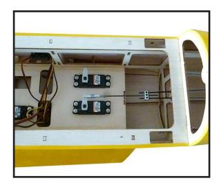
RUDDER PUSHROD HORN INSTALLATION.
