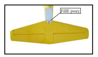
$\Box$  2) Slide the vertical stabilizer back in place. Using a triangle, check to ensure that the vertical stabilizer is aligned 90° to the horizontal stabilizer.
