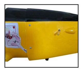
Because of the size of the cowl, it may be necessary to use a needle valve extension for the high speed needle valve. Make this out of sufficient length 1.5mm wire and install it into the end of the needle valve. Secure the wire in place by tightening the set screw in the side of the needle valve.
