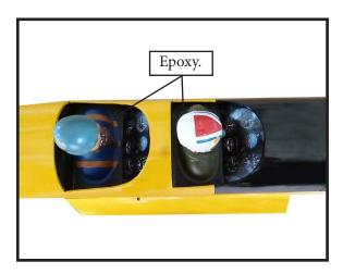
4) Epoxy canopy onto the fuselage. Trace around the canopy and onto the fuselage using a epoxy.
