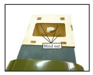
4) Attach the motor to the front of the electric motor box using four 4mm blind nut, four M4x20mm hex head bolts to secure the motor. Please see picture shown.
