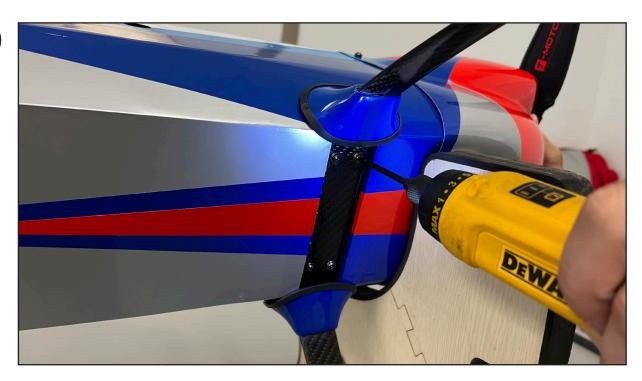
Attach the landing gear to the fuselage using screws, apply a drop of threadlocker to each screw.
