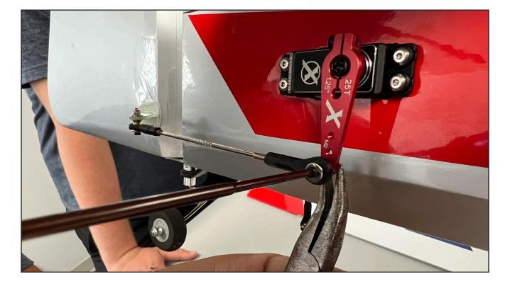
Attach the elevator pushrod as shown.
