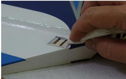
**3.** Scuff the portion of the horns that will be inserted into the elevator with sandpaper.
