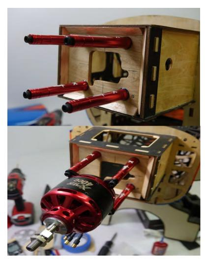
\*\*\*<u>Please note that we removed the laser scribed panels in the F1 former in our electric powered</u> airframe to allow cooling air to reach the batteries\*\*\*
