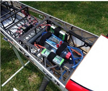
30. Mount your ignition to the interior side of the motor box lid and secure the lid with 4 screws. Next use a rotary tool to cut the cowl to clear the cylinder head, mufflers and make an air exit. <u>Take a minute</u> to add some thick CA or Epoxy to the intersection of the cowl and plywood cowl ring.
