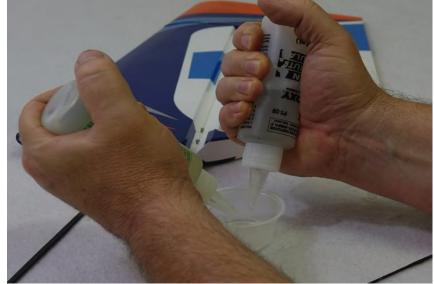
6. Use the nylon cable tie to apply epoxy to the slots and thoroughly coat the control horns on both sides of each horn.
