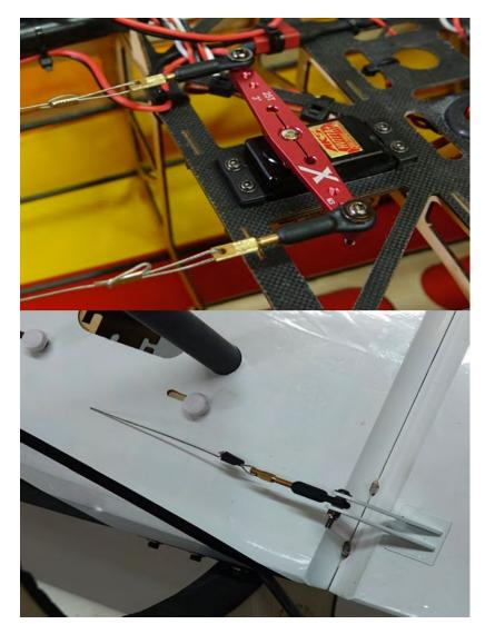
26. If using a 60cc engine or large electric motor with high capacity LiPo batteries mount the rudder servo in the provided location in the rear of the fuselage with the output spline mounted toward the rear of the aircraft. You will need to mount your rudder linkage to the interior side of the servo arm for sufficient clearance as shown. A 1.5 inch servo arm will provide full rudder deflection with travel control turned up in your transmitter menu.
