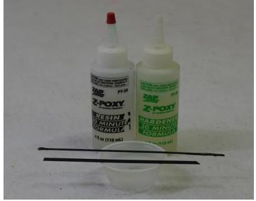
5. Mix a generous batch of epoxy being careful to use equal parts resin and hardener.
