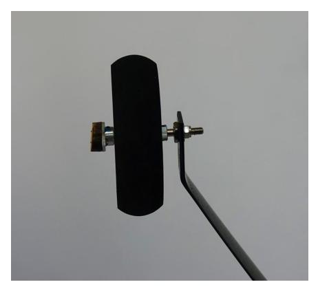
17. Slide the wheel pants into position and secure with 2 3mm bolts and washers inserted through the carbon gear and into the blind nuts in the wheel pants. Be sure to use thread lock on the bolts! Pull the pant back from the plywood support block and run a bead of Epoxy on the plywood surface to adhere the block to the wheel pant wall. This adds an enormous amount of strength and rigidity to the wheel pant.
