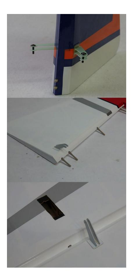
10. Assemble and install the servo mounting grommets. Connect an EF 20 AWG servo extension to each aileron servo lead (secure with heat shrink tubing or an EF Servo Safety Clip) and install the elevator and aileron servos in their designated locations. We highly recommend using the Extreme Flight socket head servo screws to mount your servos. The servo output spline of the elevator and aileron servos should be oriented toward the front of the model.
