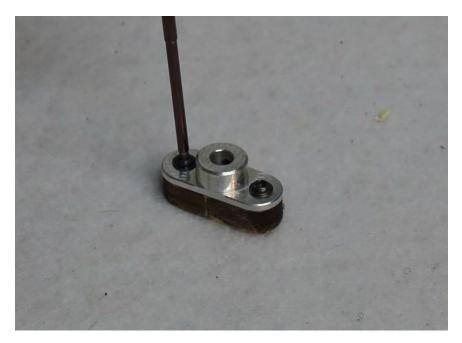
16. slide a wheel collar onto the axle followed by the wheel and then the wheel pant support. Push the wheel pant support as far as possible onto the axle and tighten the set screw, then adjust the wheel collar position to properly position the wheel on the axle as shown.
