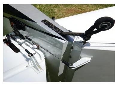
27. If you plan to keep your stabs attached to the fuselage during transport then a 36" 20 Awg servo extension is long enough. If you plan to remove the stabs you will need to use a 48" extension. Secure the extension to the elevator servo lead with an EF Servo Safety Clip or heat shrink tubing.
