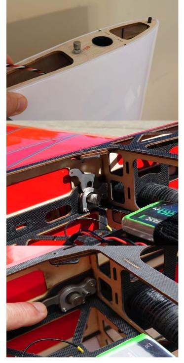
36. Included with your MXS are a set of Side Force Generators (SFGs) along with 2 clear spacers to be installed between the SFGs and wing tip to prevent them from interfering with aileron movement. They are to be installed using the supplied white thumb screws threaded through the holes in the SFG, through the clear spacer and into the pre-installed blind nuts in the wing tip.
