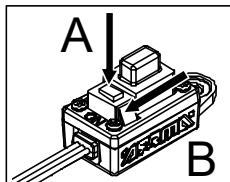
1. Connect a battery. Press and hold the set button and turn on ESC. The RED LED will flash.
