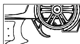
3. Throttle trigger in full brake position - press set button (3 Green flashes)
