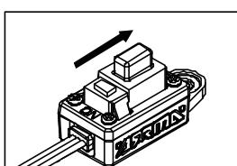
5. To save the setting, switch the ESC off. Restart the process to make more changes.
