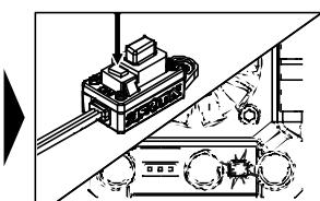
4. Using the tuning chart, press the 'set' button until the number of red LED flashes and short beeps equals the required value.
