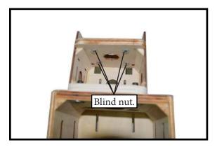
5) Attach the motor to the front of the electric motor box using four 4mm blind nut, four M4x20mm hex head bolts to secure the motor. Please see picture shown.
