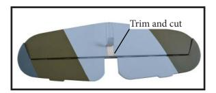
When cutting through the covering to remove it, cut with only enough pressure to only cut through the covering itself. Cutting into the balsa structure may weaken it.
