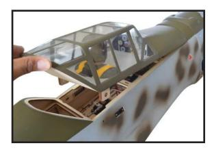
3) Position the pilot figure on the canopy floor as shown. Use epoxy to glue the base of the pilot figure to the cockpit floor, please see pictures as shown.
