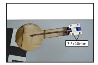
2) Install servo for Retractable landing gear.
