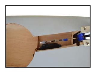
3) Secure the landing gear doors to the landing gear struts.
