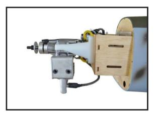
8) Reinstall the servo horn by sliding the connector over the pushrod wire. Center the throttle stick and trim and install the servo horn perpendiular to the servo center line.
