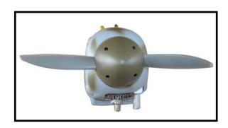
The propeller should not touch any part of the spinner cone. If it does, use a sharp modeling knife and carefully trim away the spinner cone where the propeller comes in contact with it.
