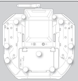
Gently remove the rear case, without pulling excessively on the wiring.
