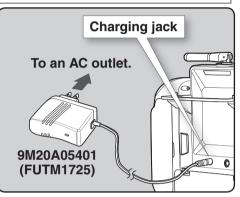
The charging time when charging the FT2F2100BV2 battery with the optional special charger is approximately 3 hours.
