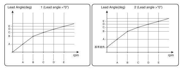
When using in races in which the lead angle setting function is inhibited by the ESC, set "Lead angle use" to "INH". The "Lead angle use" setting has priority over "Turbo mode". If "Lead angle use" is set to "INH", the lead angle setting function can be turned off even if "Turbo mode" is set to "Turbo 1" or "Turbo 2". The MC940,960CR shows that the lead angle setting function is OFF ("0" timing) by blinking a LED.
