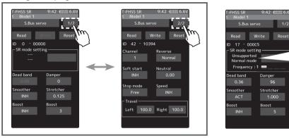
When the connected servo type is not compatible with the SR mode, "Unsupported Normal mode" is displayed
