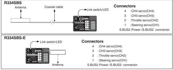
The receiver power supply can be connected to the S.BUS2 connector or each of CH1-4.
