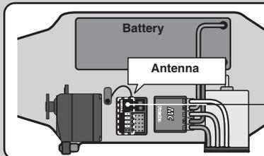
Install the receiver as far away as possible from the battery, motor controller, motor, silicon cord and other noise sources. Keep it away from the antenna wire, in particular. The example in the figure is for R404SBS.
