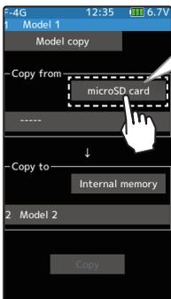
Tap to select the model of the T10PX main body or the model inside the SD card.
