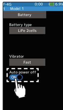
Example: When turning off the auto power-off function on the battery setting screen, tap (ON) of auto power off to display (OFF), and the function will be invalid.
