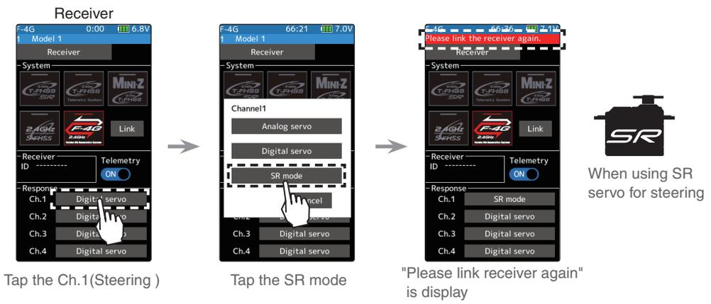
**Note:** In SR mode ON, normal servo, ESC, and standard gyro will not operate.
