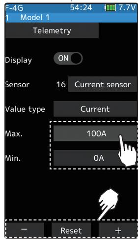
Tap the value button of the [Max.] and [Min]. Value input buttons appear on the screen. Use the [+] and [-] buttons to adjust the upper limit and lower limit amount.
