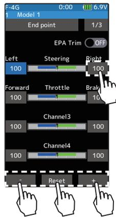
Example: To change the right-hand side steering amount on the End point screen, tap the right of the steering wheel, and when [-] [reset] [+] is displayed at the bottom of the screen, press + To decrease, tap [-] to change the numerical value. If you leave it tapped, the value changes continuously. Tap [Reset] to return to the initial value.
