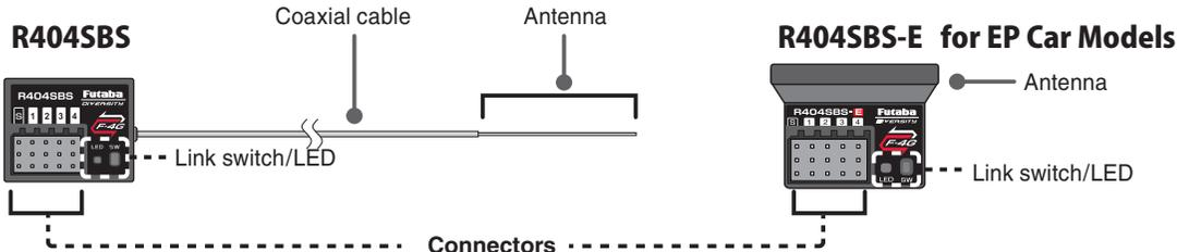
The receiver power supply can be connected to the S.BUS2 connector or each of CH1-4.
