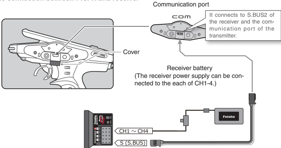
Turn on the DSP or PWR switch of T10PX and display the receiver update screen.
