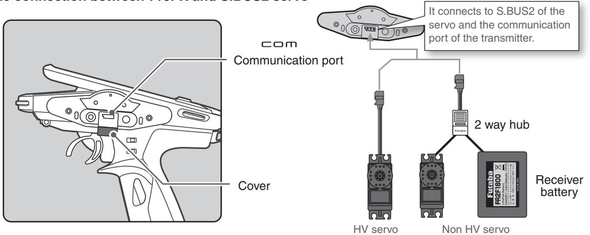
Turn on the DSP or PWR switch of T10PX and display the receiver update screen.
