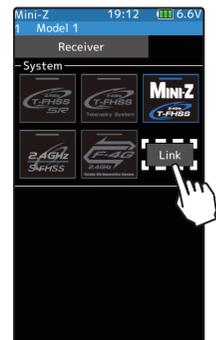
**3** Push the receiver side push switch for about 2-seconds or more.
