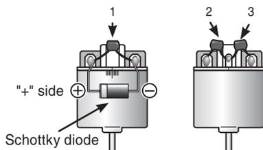
Motors with no suppressor capacitors, or inadequate suppression, may cause the receiver to malfunction. Always solder the capacitors supplied to your motor.
