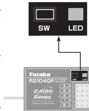
When the link is complete, the LED in the receiver changes to solid green. Check the operation of the servo.
