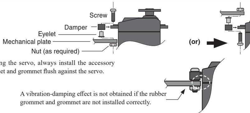
When installing the servo, always install the accessory rubber grommet and grommet flush against the servo.
