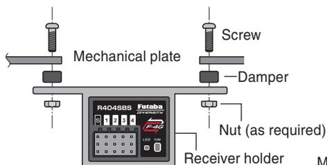
When using the receiver holder supplied with the kit, install the receiver through a rubber grommet.
