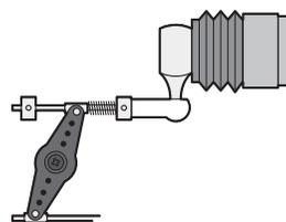
If the brakes overheat while running, their ability to function properly decreases. Before running, adjust the suitable maximum servo travel so that unreasonable force is not applied even when the servo travel is increased while running.
