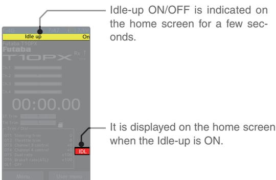
If the power switch is turned on while the Idle-up switch is on, an audible alarm will be heard. Immediately set the Idle-up switch to OFF.
