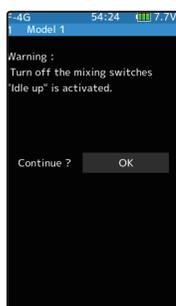
When the power switch is turned on while the idle-up, engine cut, or neutral brake function switch is on, an audible alarm will sound, and "Warning" will be displayed on the LCD. When that function switch is turned off, the alarm will stop.
