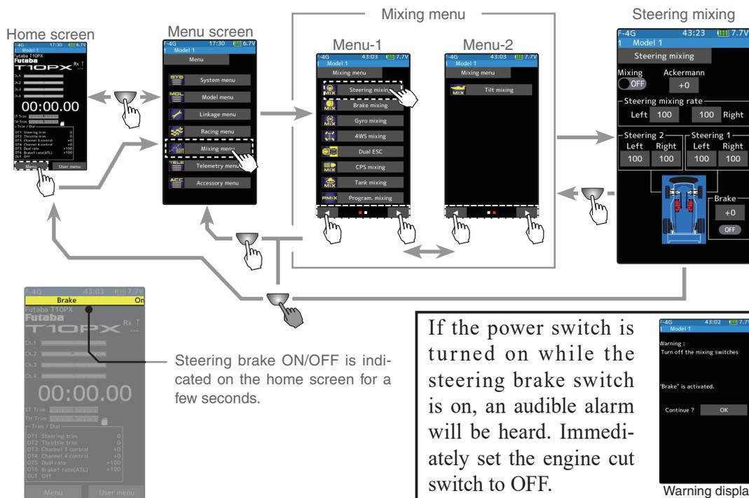
The mixing function is assigned to auxiliary channels used by another mixing cannot be used. When the number of channels is insufficient, cancel the other mixing.
