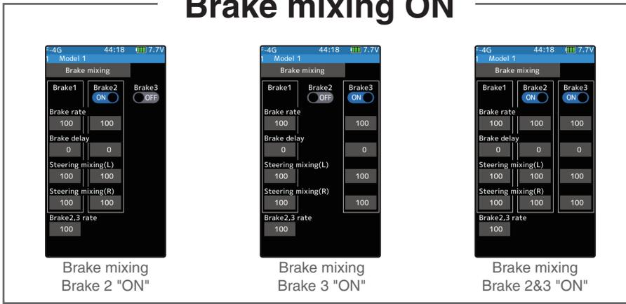
The mixing function is assigned to auxiliary channels used by another mixing cannot be used. When the number of channels is insufficient, cancel the other mixing.
