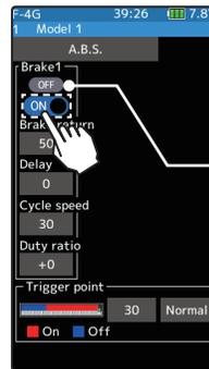
\* Displays ON/OFF of the condition that ABS is working by throttle trigger operation.
