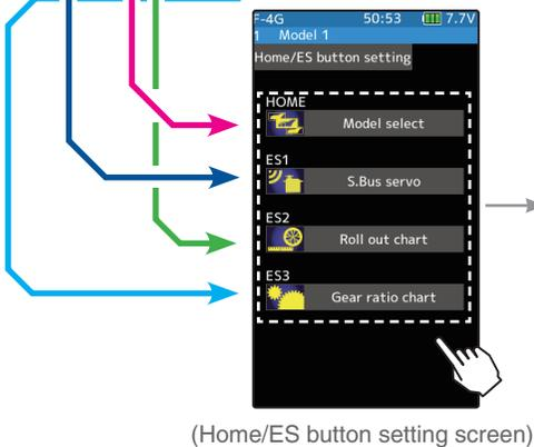
Select a screen to display by pressing ES1 - ES3 button. You can select the display of a specific function screen. Tap from the function list and select it.
