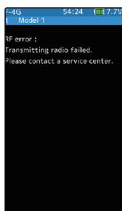
When the RF module does not operate, "RF Error" is displayed on the LCD and an audible alarm will sound. Immediately turn off the power.
