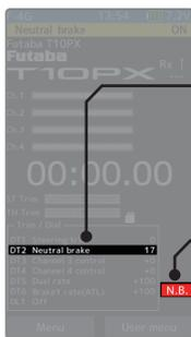
When the neutral brake is ON, the display of the throttle trim on the home screen becomes the neutral brake.
