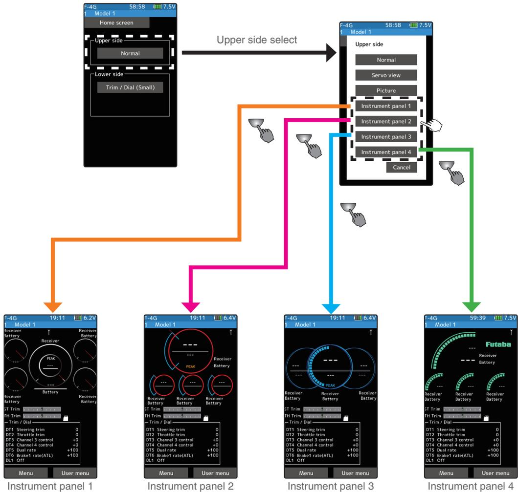
Telemetry data can be displayed on each meter.
