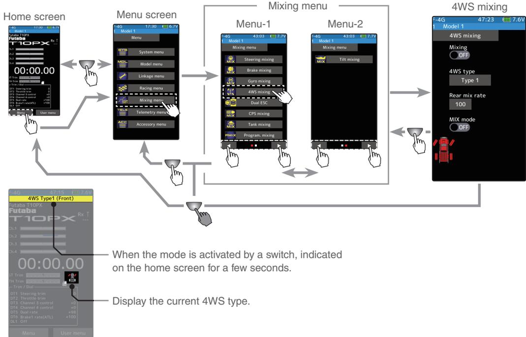
The mixing function is assigned to auxiliary channels used by another mixing cannot be used. When the number of channels is insufficient, cancel the other mixing.
