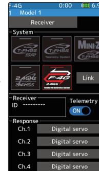
**2** In "Receiver", select and tap the system to be set from systems. The confirmation screen will be displayed. To execute, tap [Yes] to hear an electronic sound and finish setting. To cancel, select [No] and touch it. If you change the system, be sure to link it with the receiver and turn the power on again.
