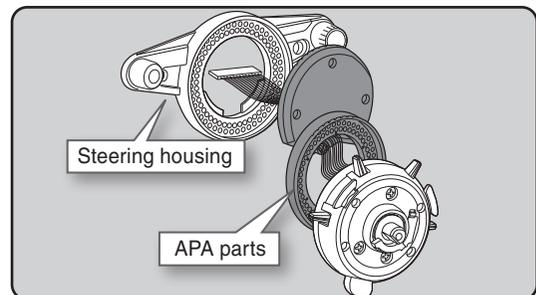
**8** Fit the rear cover and attach the APA to the steering housing with three M2x10 screws and one M2x6 screw.
