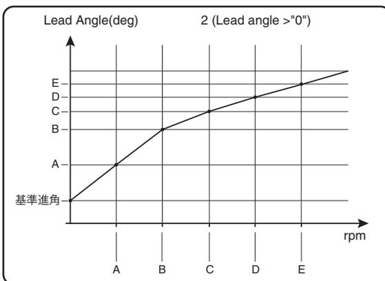
When being used while racing, the ESC inhibits the lead angle function, set "Lead angle use" to "INH". The "Lead angle use" setting has priority over "Turbo mode". If "Lead angle use" is set to "INH", the lead angle setting function can be turned off even if "Turbo mode" is set to "Turbo 1" or "Turbo 2".
