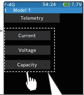
In the case of a current sensor, for example, it is possible to select from current/voltage/consumption capacity, to select data to display from a plurality of data. It is also possible to display all three data with separate meters.
