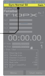
When changing the gain with the switch, indicated on the home screen for a few seconds.
