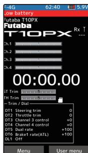
If the transmitter battery voltage drops below the usable range, an audible alarm will sound and "Low battery" will be displayed. Since the usable range of LiPo, LiFe and Ni-MH batteries are different, the power supply used must be set by the system setting.
