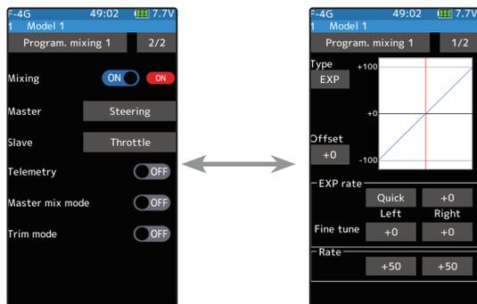
On page 1, the setting screen such as the curve, mixing rate adjustment screen, page 2, mixing ON/OFF, etc. is displayed.
