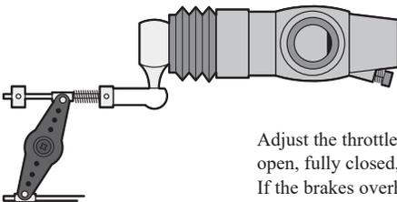
Adjust the throttle servo so that unreasonable force is not applied when the engine carburetor is fully open, fully closed, and the brakes are implemented fully. If the brakes overheat while running, their ability to function correctly decreases. Before running, adjust the suitable maximum servo travel so that unreasonable force is not applied even when the servo travel is increased while running.
