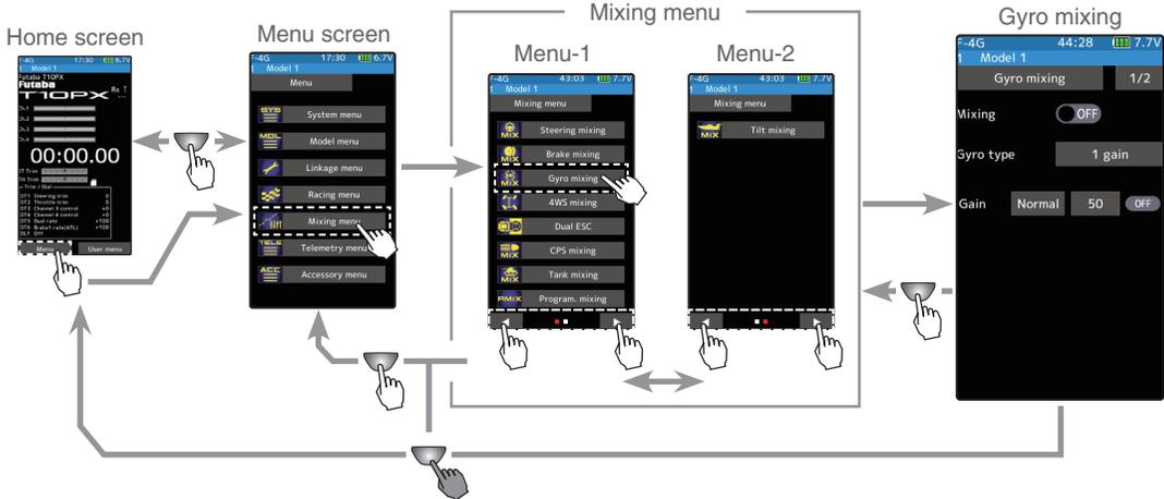
The mixing function is assigned to auxiliary channels used by another mixing cannot be used. When the number of channels is insufficient, cancel the other mixing.
