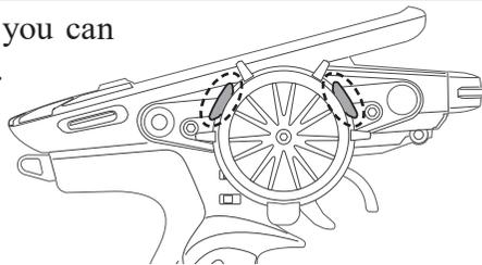
**1** Remove the wheel unit from the transmitter according to "Installing the accessory APA steering wheel offset adapter".
