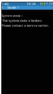
If the data is lost for an unknown reason, an audible alarm will sound, and "System error" will be displayed on the LCD screen.
