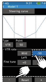
To set the right and left steering curves separately, tap the rate in the direction you wish to change the setting. Value input buttons appear on the screen, use the [+] or [-] buttons to adjust the steering curve.
