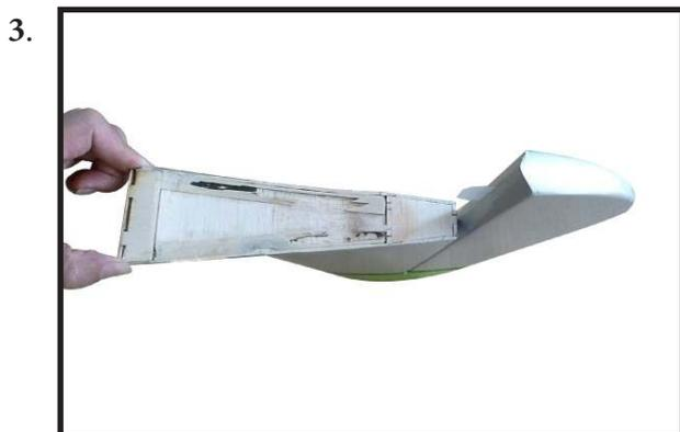
Slide the vertical stabilizer into the slot in the top of the fuselage. The rear edge of the stabilizer should be flush with the rear edge of the fuselage and the lower rudder hinge should engage the precut hinge slot in the lower fuselage. The bottom edge of the stabilizer should also be firmly pushed against the top of the horizontal stabilizer.
