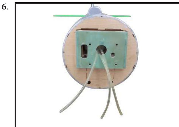
Connect the lines from the tank to the engine and muffler. The vent line will connect to the muffler and the line from the tank to the carburetor.
