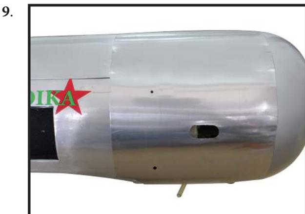
Install the muffler and muffler extension onto the engine and make the cutout in the cowl for muffler clearance. Connect the fuel and pressure lines to the carburetor, muffler and fuel filter valve. Secure the cowl to fuselage using the M3x10mm socket head screws. Putting a small length of silicon fuel tube under the head of the screw helps with vibration.
