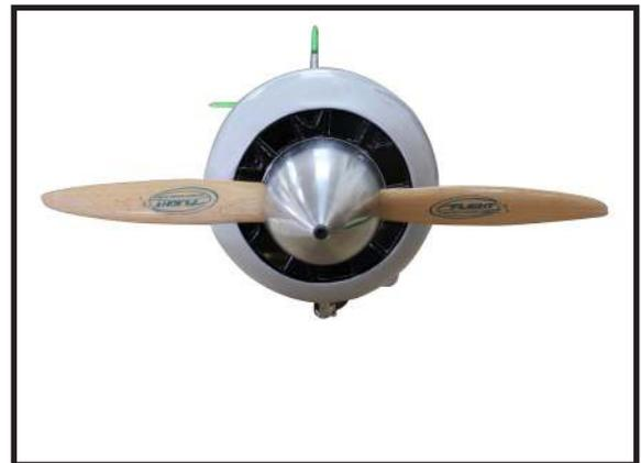
⚠ The propeller should not touch any part of the spinner cone. If it does, use a sharp modeling knife and carefully trim away the spinner cone where the propeller comes in contact with it.
