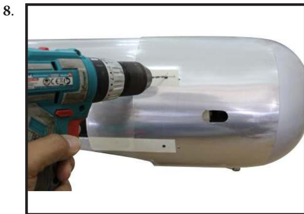
With the muffler, needle valve, and spark/ glow plug removed from the engine, slide the cowl in place over the engine. Temporarily install the propeller and spinner in order to find the exact location of the cowl. When satisfied with the cowl placement, secure the cowl to the fuselage using masking tape.
