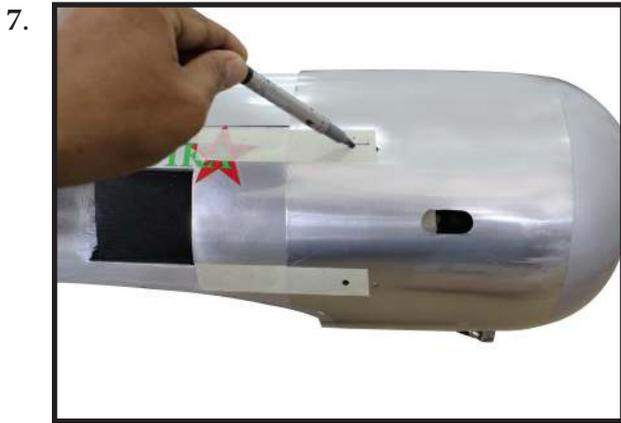
Use a drill and drill bit to drill the holes for the cowl mounting screws. Make sure the cowl position is correct before drilling each hole.
