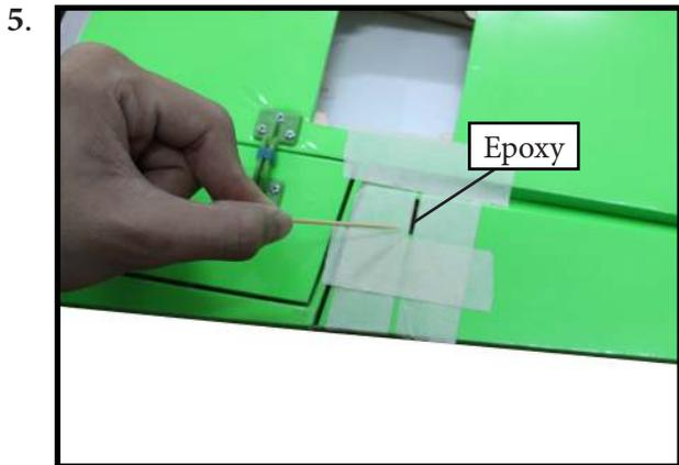
Apply epoxy to the area of the control horns that fit into the slots. Use enough epoxy so the control horns will be fully bonded to the fixed surfaces.
