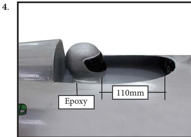
Epoxy canopy onto the fuselage. Trace around the canopy and onto the fuselage using a epoxy.
