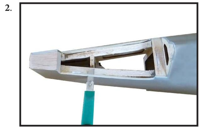
Slide the stabilizer into place in the precut slot in the rear of the fuselage. The stabilizer should be pushed firmly against the front of the slot.
