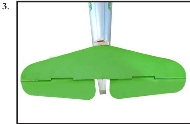
With the stabilizer held firmly in place, use a pen and draw lines onto the stabilizer where it and the fuselage sides meet. Do this on both the right and left sides and top and bottom of the stabilizer.
