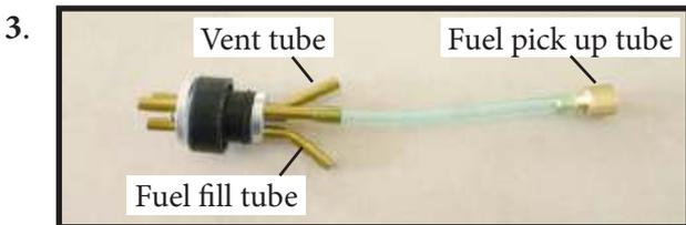
Carefully bend the second nylon tube up at a 45° angle. This tube is the vent tube.
