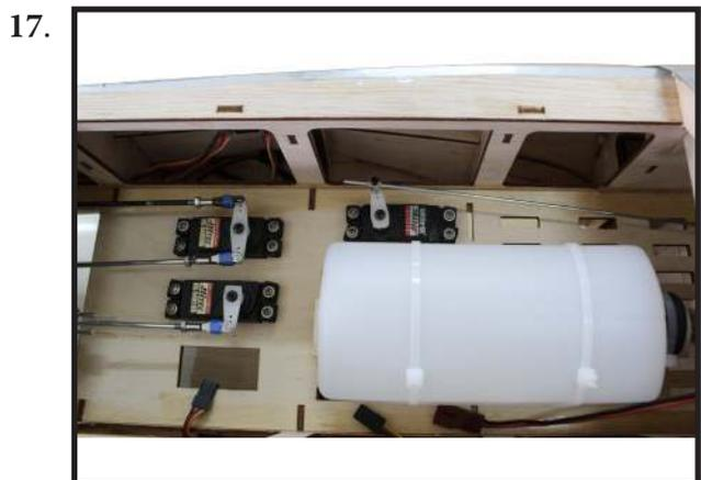
Reinstall the servo horn by sliding the connector over the pushrod wire. Center the throttle stick and trim and install the servo horn perpendicular to the servo center line.
