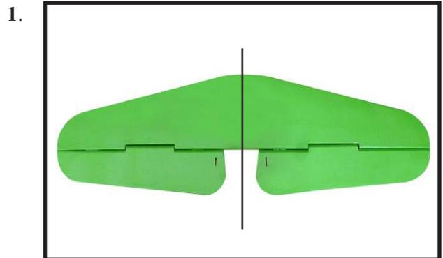
Using a modeling knife, carefully remove the covering at mounting slot of horizontal stabilizer ( both side of fuselage).
