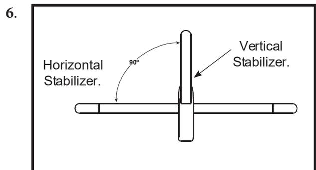
Slide the vertical stabilizer back in place. Using a triangle, check to ensure that the vertical stabilizer is aligned  $90^\circ$  to the horizontal stabilizer.
