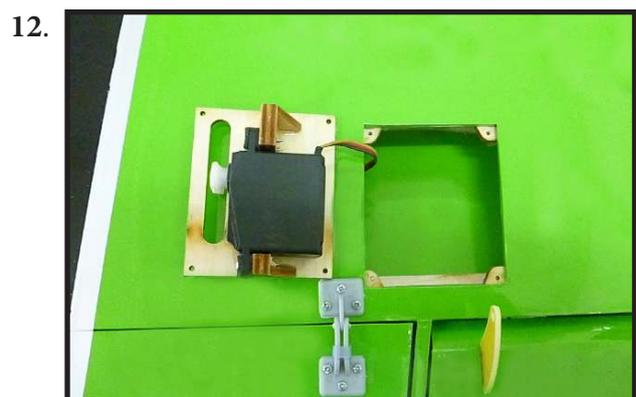
Set the aileron hatch in place and use a Phillips screw driver to install it with four wood screws.
