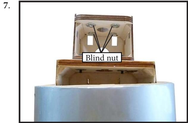
Attach the motor to the front of the electric motor box using four 4mm blind nut, four M4x20mm hex head bolts to secure the motor. Please see picture shown.
