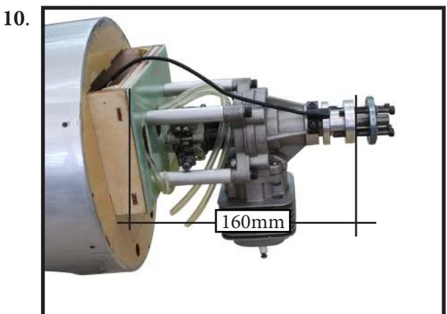
Position the engine with the drive washer (160mm) forward of the firewall.
