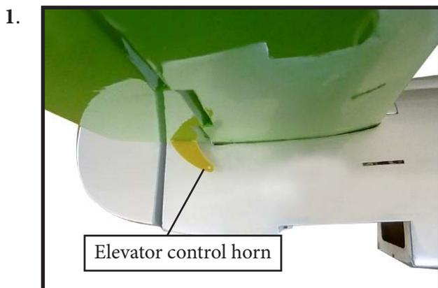
Thread one clevis and M2 lock nut on to each elevator control rod. Thread the horns on until they are flush with the ends of the control rods.
