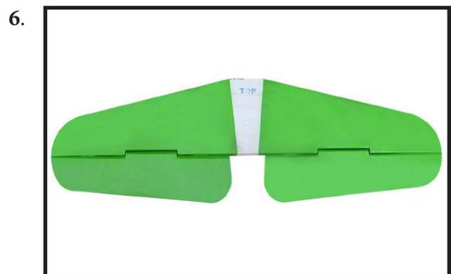
When you are sure that everything is aligned correctly, mix up a generous amount of 30 Minute Epoxy. Apply a thin layer to the top and bottom of the stabilizer mounting area and to the stabilizer mounting platform sides in the fuselage. Slide the stabilizer in place and realign. Double check all of your measurements once more before the epoxy cures. Hold the stabilizer in place with T-pins or masking tape and remove any excess epoxy using a paper towel and rubbing alcohol.
