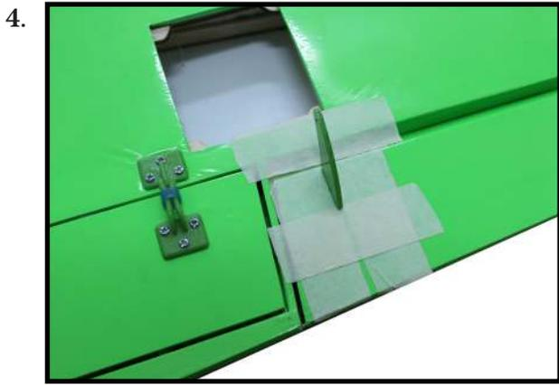
Remove the control horns from the control surfaces. Apply epoxy to the slot in the aileron and flap. Make sure the epoxy gets into the slot for a good bond between the surfaces and control horn.
