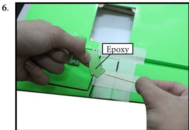
Before the epoxy fully cures, remove the tape from around the control horn. This will allow the epoxy to flow around the control horn, creating a small fillet between the control horn and surface for a finished look and secure bond.
